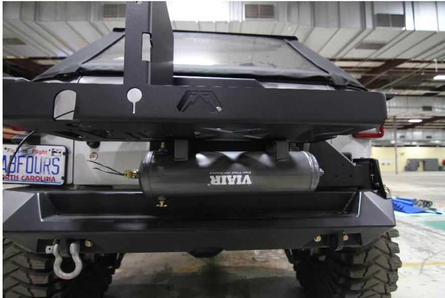
Figure 1: Air Tank Installation
