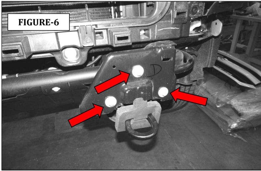
**Step-8** If equipped, using a 18mm socket, ratchet and wrench remove the nut and (2) bolts' securing the tow hooks to the frame, (FIGURE-7). Note: The tow hooks will not be reinstalled.
