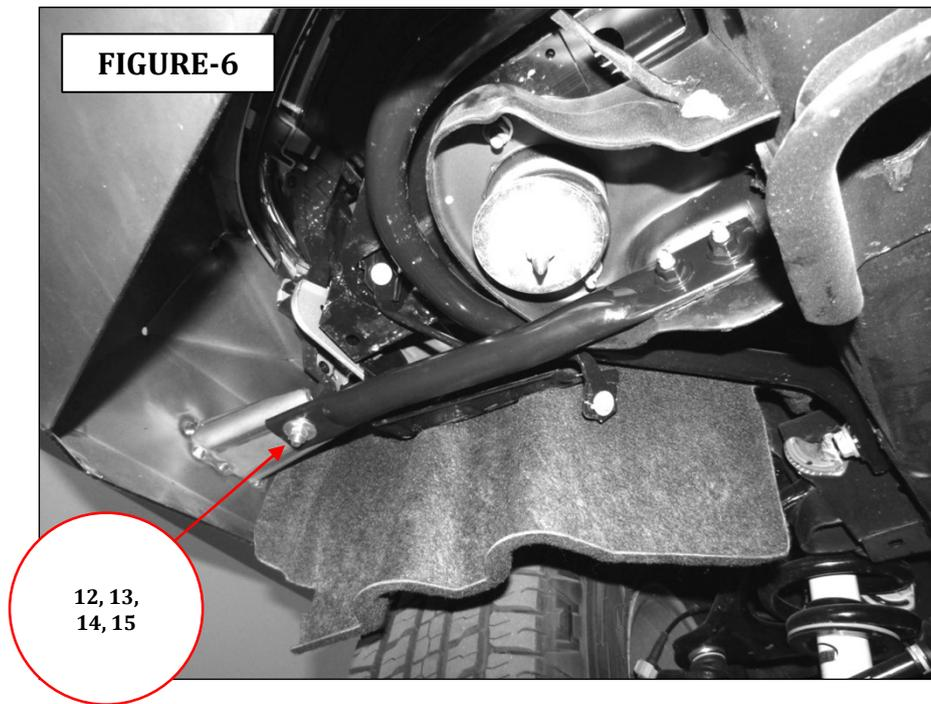
**Step-8** With assistance, adjust and hold the bumper shell visual alignment position, then tighten all factory and supplied nuts and bolts securing the brackets, winch tray and bumper shell.
