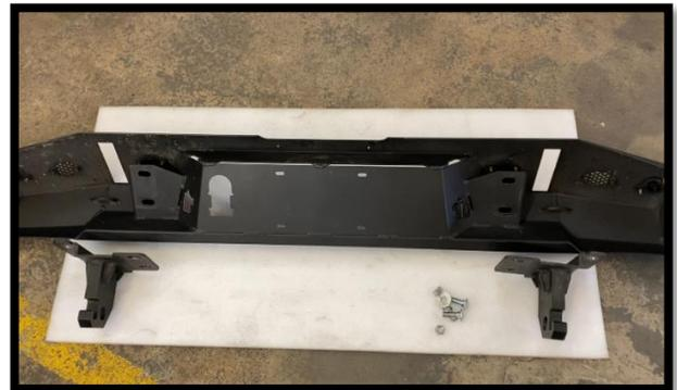
Lay bumper on a protective surface to prevent finish from damage. You'll need to preassemble the rear brackets onto the bumper. Determine where each bracket goes on the backside of the bumper.
