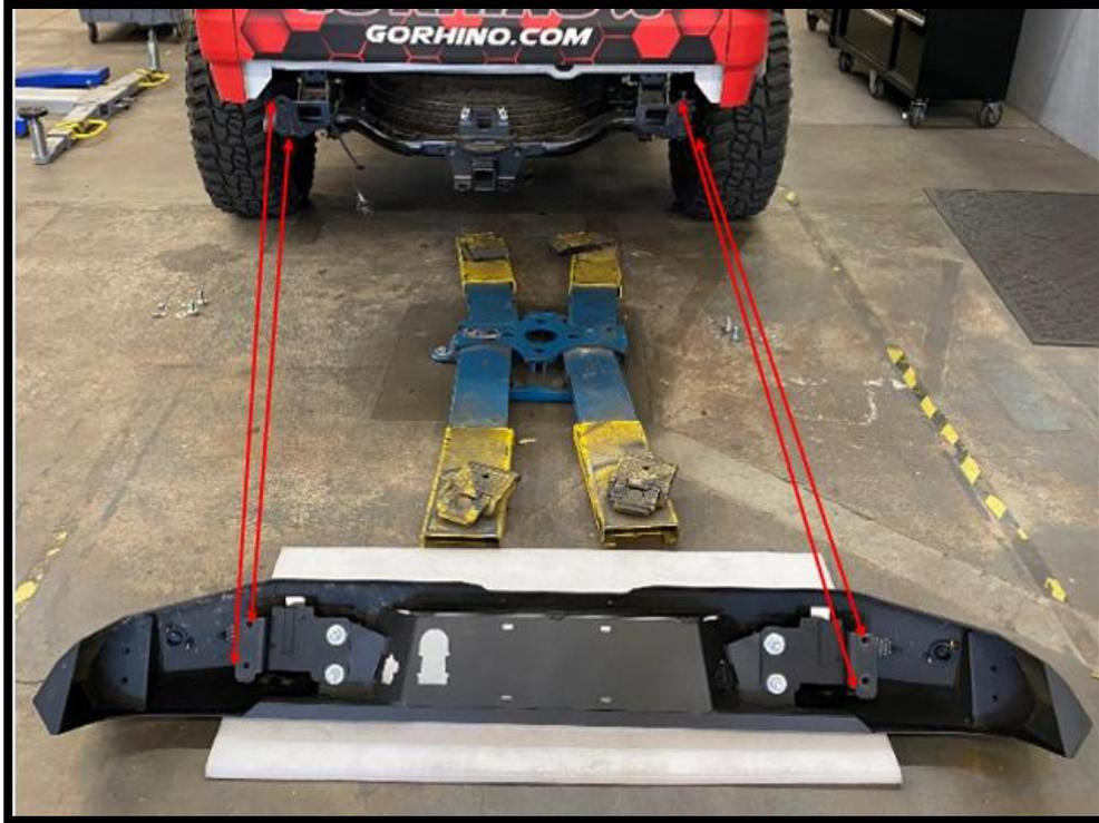
With assistance, position bumper onto OEM bumper mounts.
