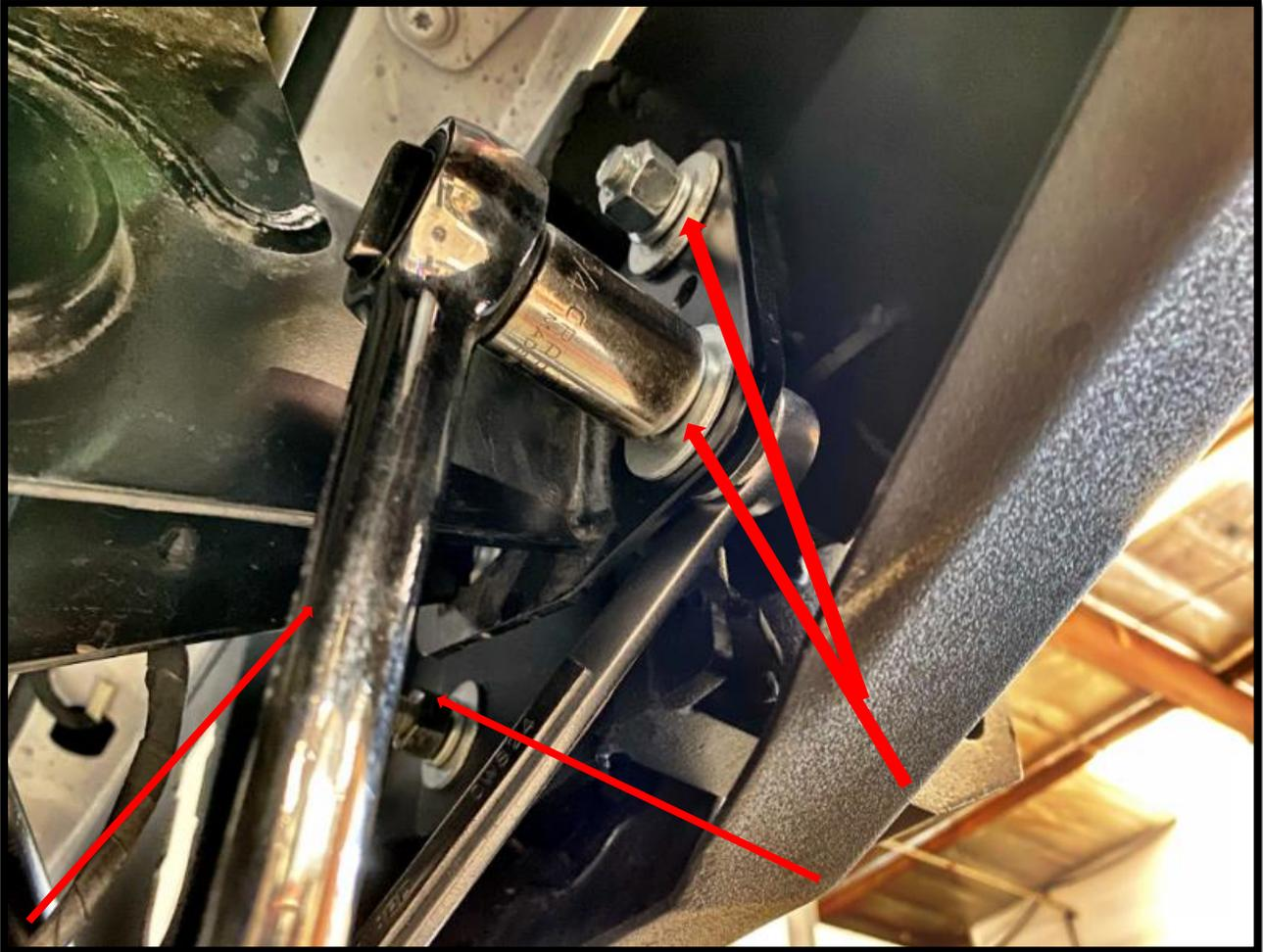
Begin to fasten ½" hardware with ¾" wrench or socket. Be sure to fasten all four nuts (4 per side). Begin to align bumper to square up with the bed.
