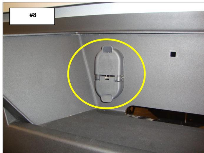
**Step-12** Reconnect the factory bumper wiring harness to the sensors and to the vehicle wiring harness. Note: In order to connect the wiring harness to the (2) inner sensors the wires inside the conduit will require rerouting.
