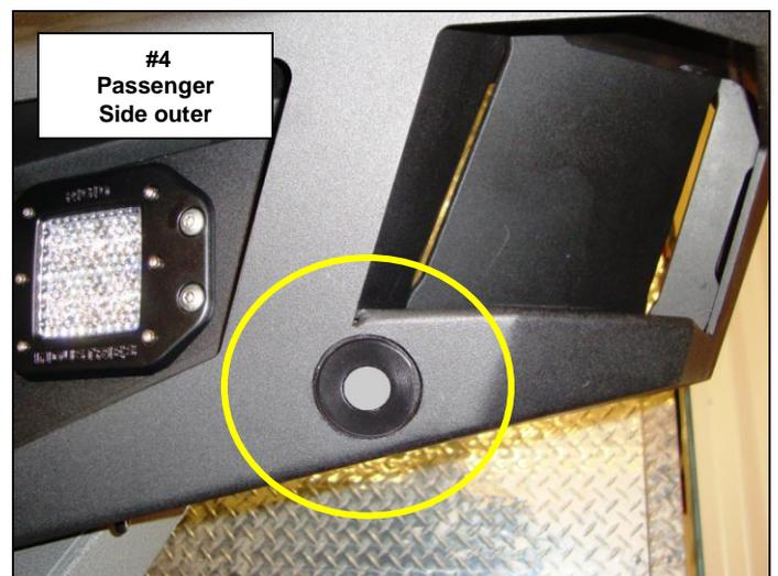
**Step-8** Remove the (2) bolts and frame plates from the driver and passenger side of the frame/receiver hitch, (Photo 5).
