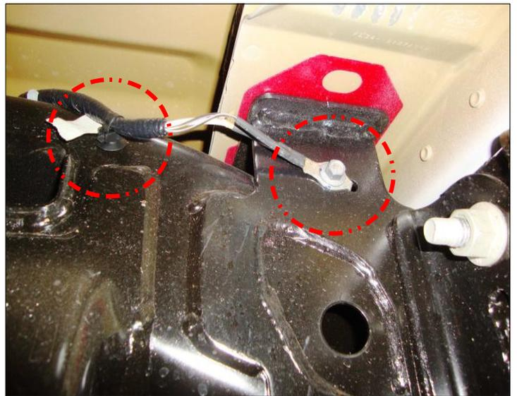
**STEP #3** With assistance support the rear bumper and remove the (3) nuts on each side of the vehicle securing the factory bumper and receiver hitch to the frame. Remove the bumper from the vehicle, (Photo 3).
