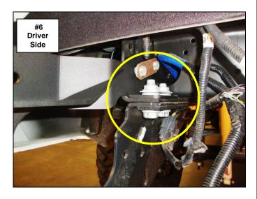
**Step-9** With assistance attach the bumper shell brackets to each frame bracket using (2) ½" x 1 ½" hex bolts, (4) ½" flat washers, (2) ½" lock washers and (2) ½" Hex nuts, (Photo 7). Align the bumper shell with the vehicle, verify that the tailgate clears when lowered, then tighten the nuts and bolt plate securing the frame bracket to the side of the frame first then tighten all remaining factory and supplied nuts and bolts.
