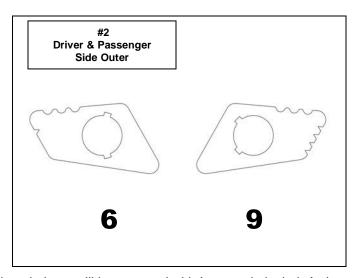
**Step-4** Prepare the inside surface of the bumper shell where the bezel plates will be mounted with Isopropyl alcohol. A clean, dry surface is required in order for tape to stick properly.
