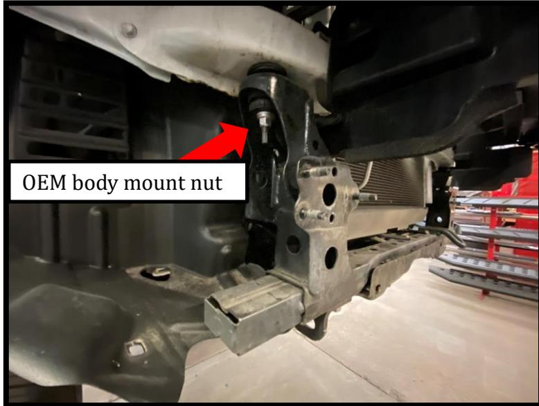
Remove OEM front body mount nut to install outer auxiliary brackets. Install auxiliary bracket in place with OEM washer in the same position. The auxiliary bracket should sandwich itself between the OEM mount washer and OEM mount nut. Refer to your OEM manual on removal process.
