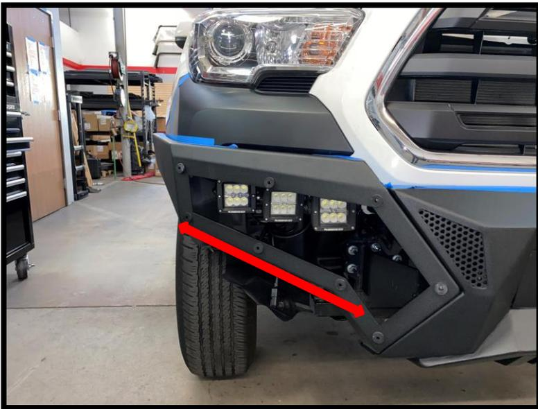
Once you have adjusted the fitment on your bumper, you can cut the fender liners. Depending on your desired look, you can cut the OEM fender liner by following the Element bumper lines. With caution, use a cutting wheel or box cutter to cut the inner fender liner. If you prefer to cut more material, please refer to the images below. You can sand the edges to so they are not left sharp.
