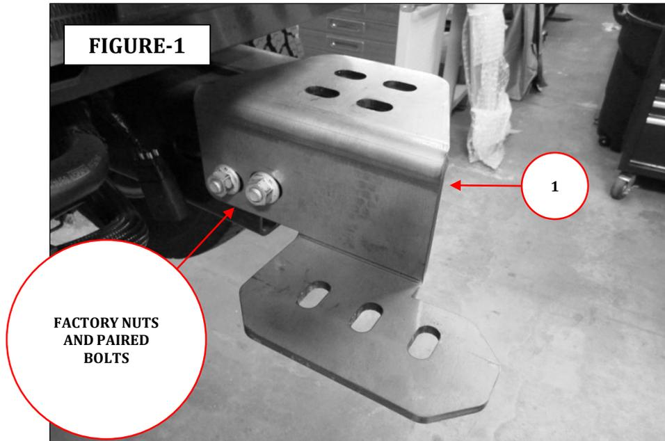
**Step-2** Install the driver's side auxiliary bracket by positioning the auxiliary bracket on top of the frame bracket, align the holes and secure the auxiliary bracket and frame bracket to the frame using (4) 1/2" x 2" hex bolts (8) 1/2" flat washers, (3) 1/2" lock washers and (4) 1/2" hex nuts. Leave the nuts and bolts loose for final adjustment, (FIGURE 2). Repeat this step to install the passenger side auxiliary bracket.
