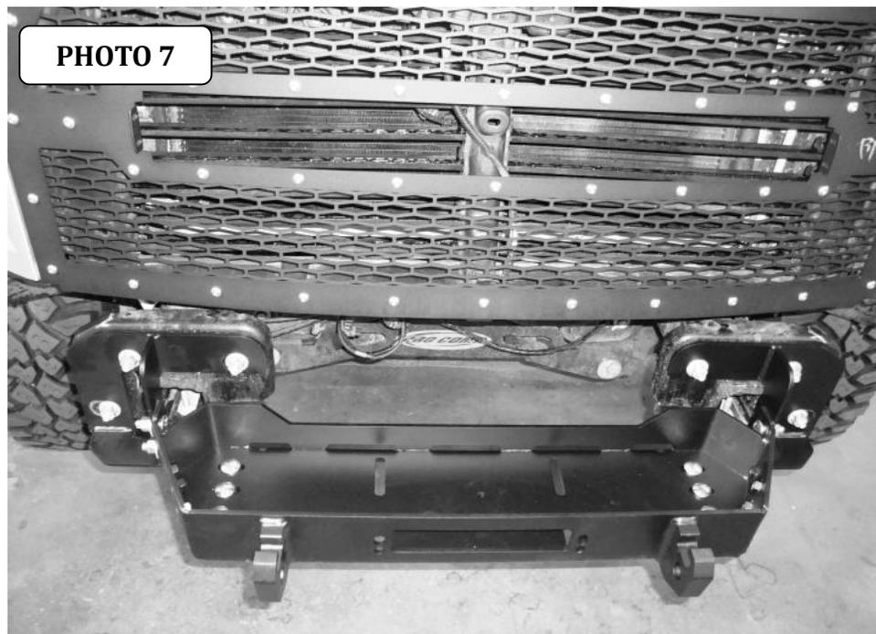
**Step-6** If you are installing a winch, place the winch in the mounting plate/winch tray and refer to the winch manufacturer's instructions for installation. Do not install the fairlead at this time.
