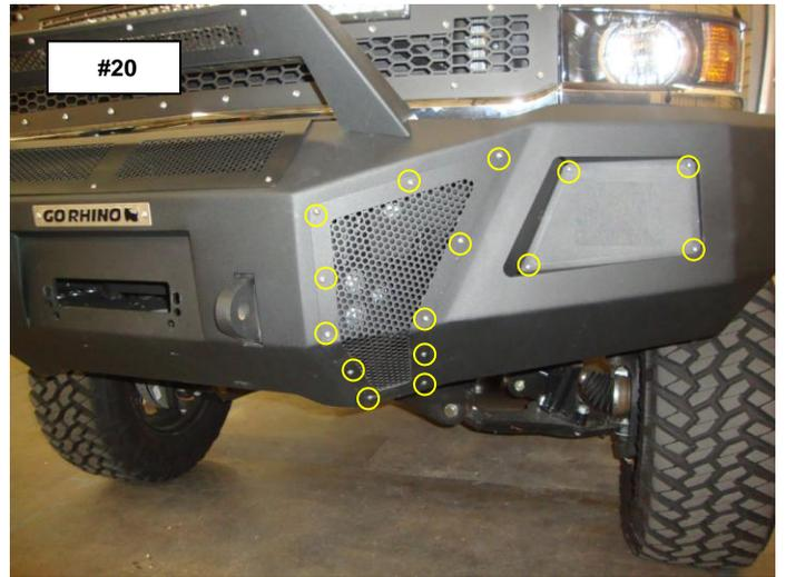
If your state law requires a front license plate, attach the license plate bracket to the holes in the face of the bumper shell, using the supplied 3/8" bolts, washers and nuts, and the license plate to the (2) obround holes in the license plate bracket using the supplied 1/4" bolts and nuts.
