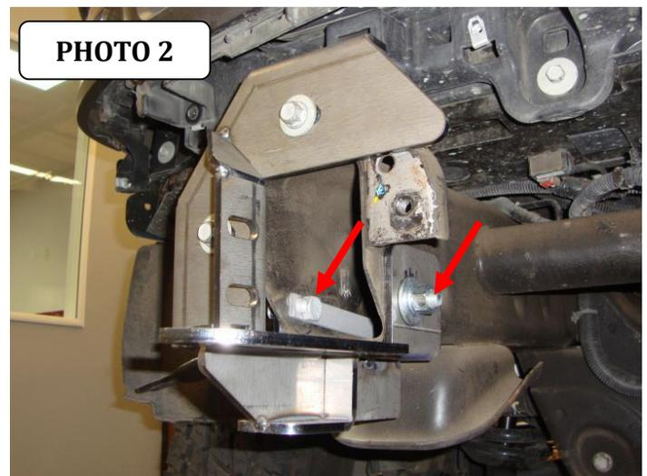
**Step-11** Position the mounting plate/winch tray on top of the auxiliary brackets. Align the holes and secure the mounting plate/winch tray to each frame bracket using (2) ½" x 1 ½" carriage bolts, (2) ½" flat washers, (2) ½" lock washers and (2) ½" hex nuts, and to each auxiliary bracket using (3) ½" x 1 ½" carriage bolts, (3) ½" flat washers, (3) ½" lock washers and (3) ½" hex nut, (Photo 3 & 4).
