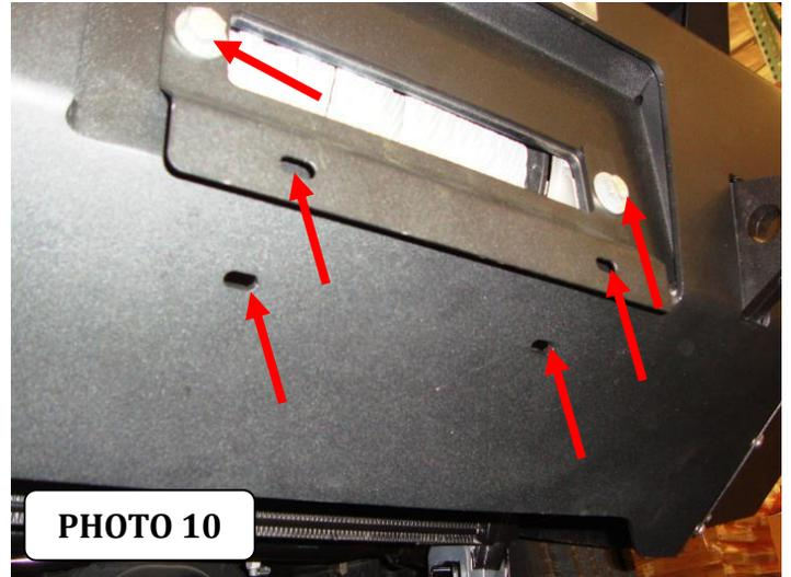
If installing a winch, attach the license plate directly to the (2) obround holes in the lower face of the bumper shell using the supplied ¼" bolts and nuts, (Photo 10).
