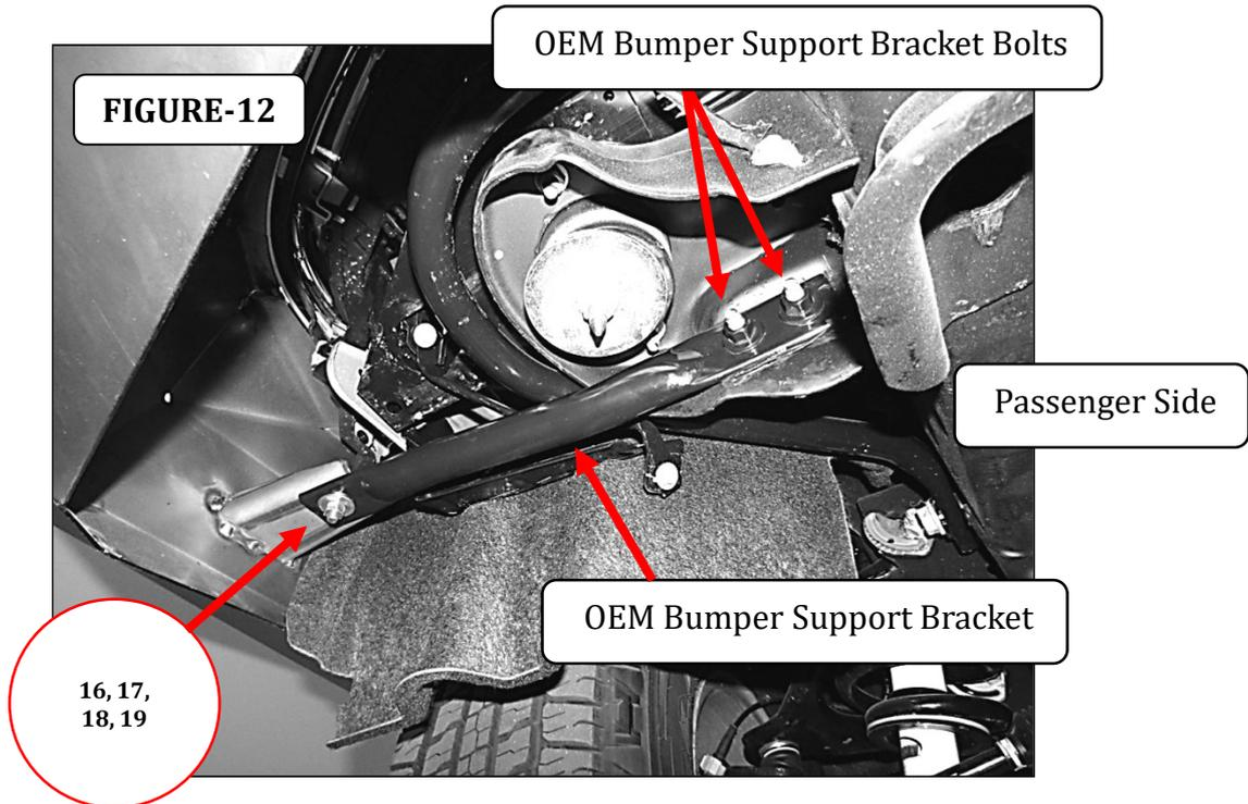
**Step-9** With assistance, adjust and hold the bumper shell visual alignment position, then tighten all factory and supplied nuts and bolts securing the brackets, winch tray and bumper shell.
