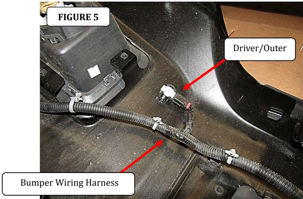
**5a** Remove each sensor from the bezel by gently spreading the bezel tabs and pulling out on the back of the sensor.
