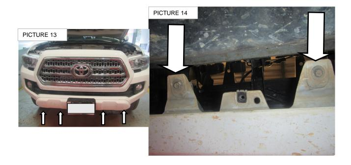
**Step-9** Remove four securing clip from bumper as indicate. (PICTURES 14 & 15)
