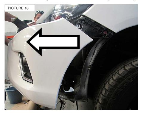
**Step-10** Pull out the sides & lower plastic cover toward out to the vehicle. This parts don't used again. (PICTURES 17)
