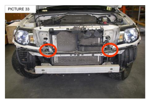
**Step-19** Remove 2 k lath screws on lower back of front grill, put the bracket grill and install the k lath screws from hardware kit (**don't tight**), re install the front gril, re install the 4 (10mm)nut. (PICTURE 34)
