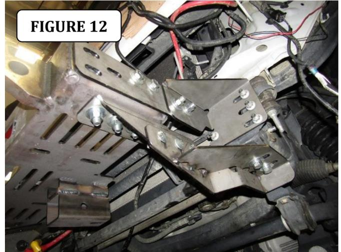
**Step-6** Position the winch tray on top of the lower extension brackets. Secure the winch tray to each upper extension bracket using (2) ½" x 1 ½" hex bolts, (2) ½" flat washers, (2) ½" lock washers and (2) ½" hex nuts, and to each lower extension bracket using (3) ½" x 1 ½" carriage bolts, (3) ½" flat washers, (3) ½" lock washers and (3) ½" hex nut, (FIGURE 12). Snug but do not fully tighten the nuts and bolts.
