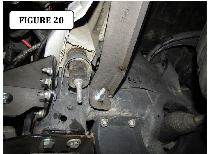
**Step-14** Secure the driver side support bracket to the frame using the T-Bolt, (1) 1/2" flat washer, (1) 1/2" lock washer and (1) 1/2" hex nut, (FIGURE 20). Attach the opposite end of the support bracket to the bumper shell bracket using (1) 3/8" x 1 1/4" hex bolt, (1) 3/8" lock washer, (2) 3/8" flat washers and (1) 3/8" hex nut, (FIGURE 21). Leave the bolts loose for final adjustment.
