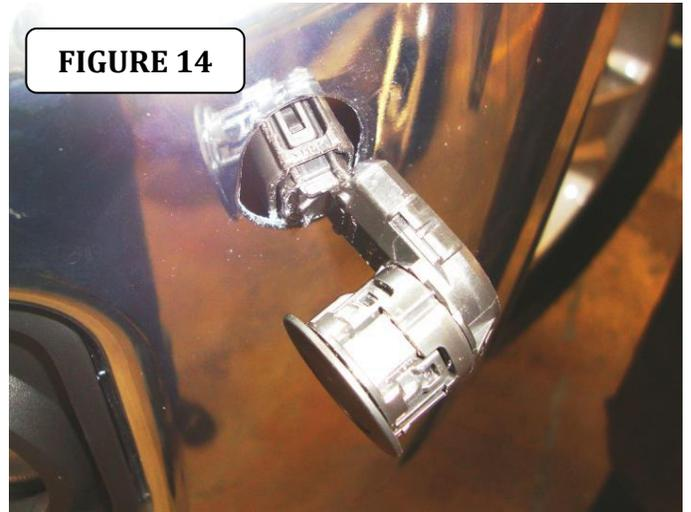
**Step-9** Remove the sensor plates that are preinstalled in the BR6 bumper. Discard the plastic plugs from the sensor plates.
