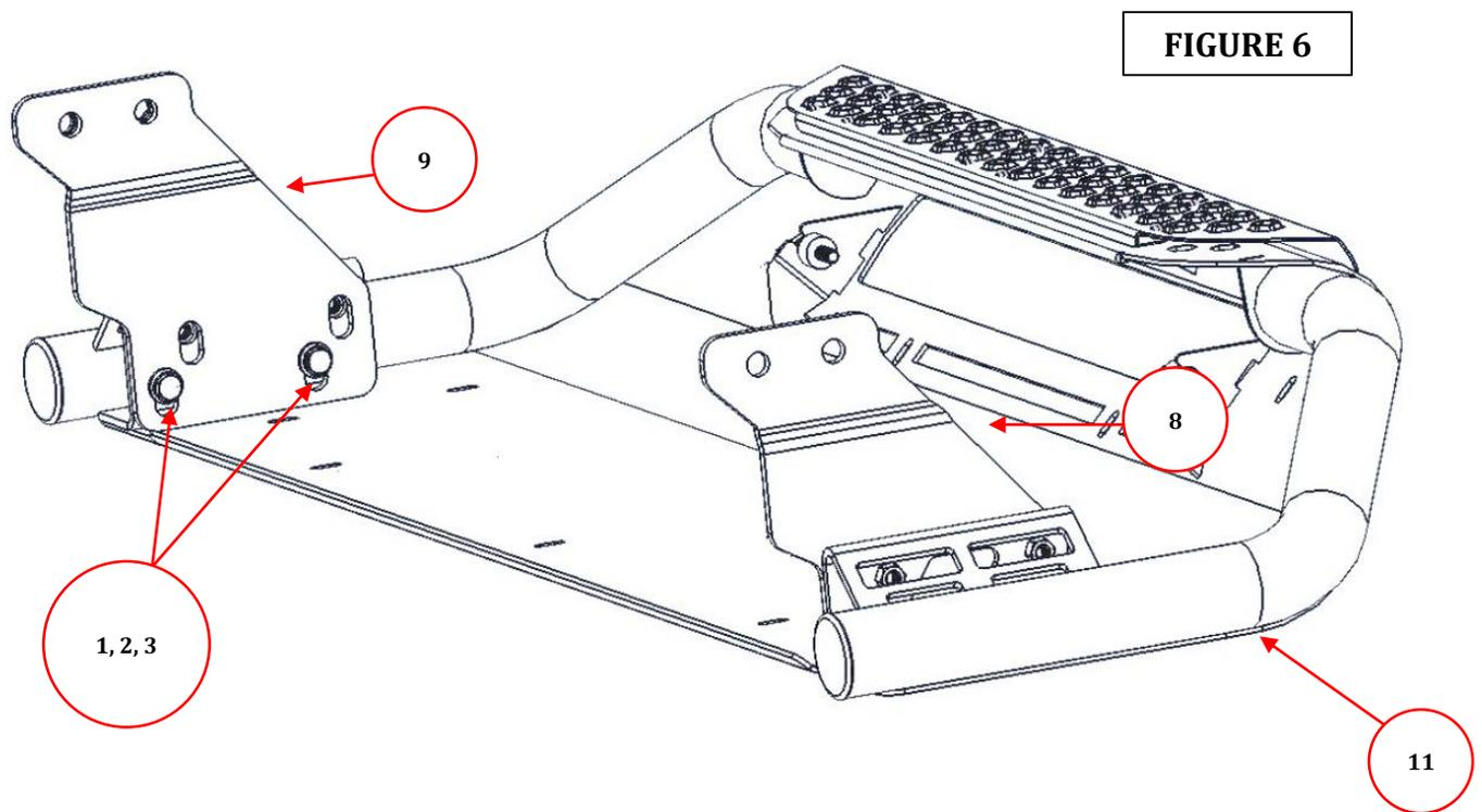
**Step-7** With assistance align and hold the RC3 front guard in the desired position on the vehicle, then tighten all OEM and supplied nuts and bolts.
