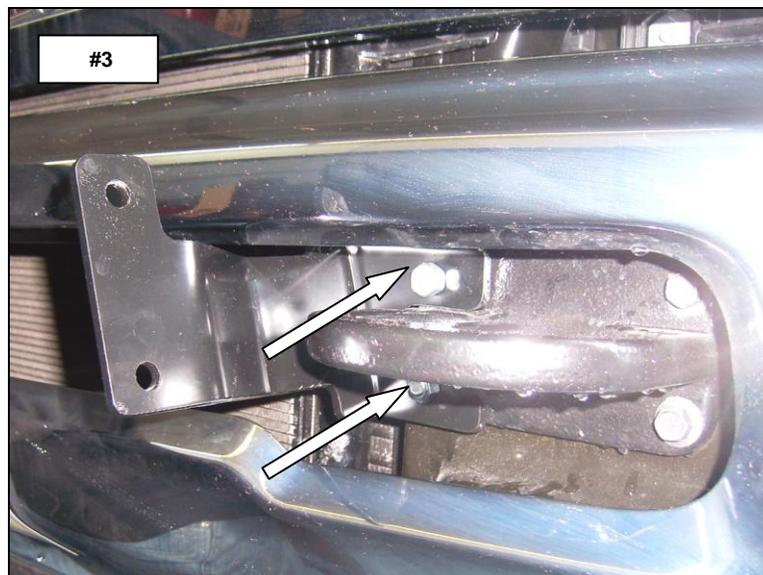
**STEP-3** POSITION THE RHINO CHARGER BULL BAR MOUNTING TABS BETWEEN THE DRIVER AND PASSENGER SIDE BRACKETS AND ATTACH THE TABS TO THE BRACKETS USING (2) 3/8" X 1" HEX BOLTS, FLAT WASHERS, LOCK WASHERS AND HEX NUTS. **PHOTO #4**
