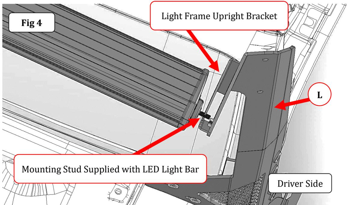
**Step-4** Attach a retainer plate to the light bar mounting stud using the fasteners included with the light bar, and attach the opposite end of the retainer plate to the light frame upright using (1) 1/4" x 3/4" button head screw, (1) 1/4" lock washer and (1) 1/4" flat washer, (Fig 5). Repeat for the passenger side.
