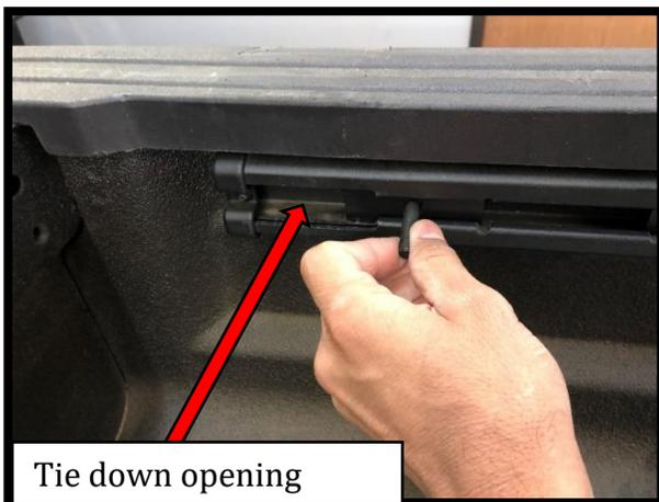
With tie down cleats removed, install Bed Track Mounting Plate with 5/16" Carriage Bolt bolt plates onto bed track system, the opening is located at the front or at the rear of the bed. Each side will use (6) bolt plate and (6) carriage bolts.
