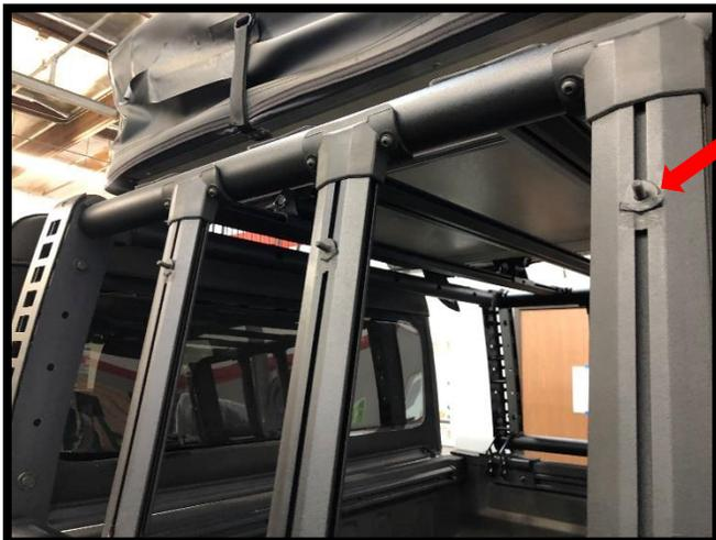
\*\*\* Installation Tip\*\*\* use painters tape to keep the bolt stationary and not sliding downwards during installation
