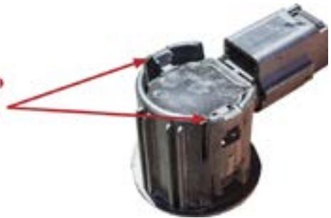
5. Carefully pull the plastic center piece of the bumper off. There are no tools required for this step, it pulls off by hand. "Fig C"
