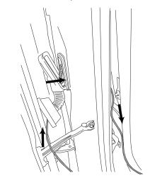
Feed wire to front sill area. Run wire between door seal and black wire casing. Place wire under loom and connect red wire to powerstep trigger wire (Light blue and black stripe on driver side and Green with a black stripe on passenger side)with supplied butt connector. Once crimped use heat gun to shrink tube.
