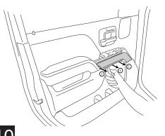
Remove Front door Cover plates behind door handle and in bottom of grab handle to access mounting
