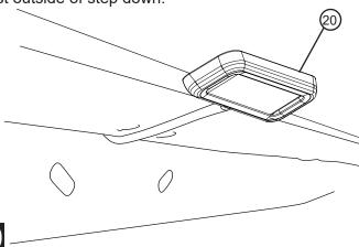
Using supplied butt connectors, connect the lamp wires. Red to Red, Black to Black. Once Crimped use heat gun to shrink tube. Close and wrap conduit with electrical tape. Secure all loose wires with cable ties. Pull lamp wires upward to avoid any wire snagging.
