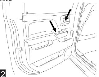
Using a 7mm socket remove the 4 screws that secure the rear door panel in place.
