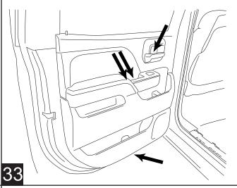
Pry all panel fasteners loose. Start at door hinge side and work your way around the bottom and towards latch side of door.
