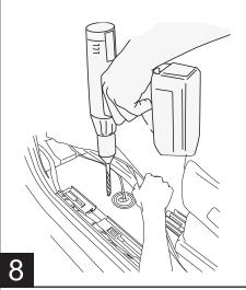
Route wire harness along the frame and back towards rear linkage. Secure with zip ties. Push both wires through rubber grommet. Connect harness to motor. Secure harness with tie wraps.
