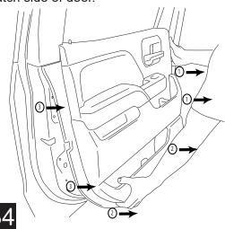
Once panel pins are out lift up on panel. Lift panel up and off of door.
