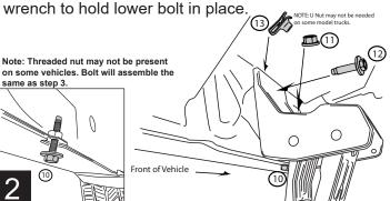
**Rear Drive Linkage:** Install driver side Motor Linkage in fourth sheetmetal tab / hole from front. Linkage will then clear parking brake cable.
