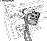
Remove power fuse. Attach power lead (RED wire) to positive pole on the battery. Attach ground lead to negative battery pole.
