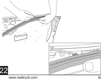
Attach clips to grooves in door.
