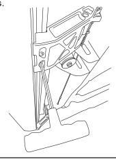
Using the two 11" cable ties, mount controller to support arm next to battery. Plug in harness (Ensure that locking tabs engage)
