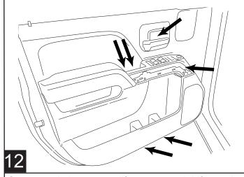
Once panel pins are out lift up on panel. Lift panel up and off of door.
