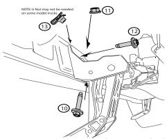
Set linkage into second to last sheetmetal tab / hole from rear. Use supplied bolt (10) and nut (11) to hold in position. Install bolt (12) into upper mounting hole and snug both bolts. Torque upper bolt (12) to 16ft-lbs (22N m) first and then torque lower bolt (10) and nut (11) to 16 ft-lb (22N m). Repeat linkage installation on Passenger side.
