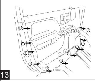
Remove door latch cable from door panel.
