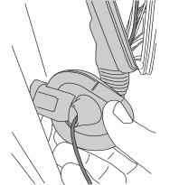
Route trigger wire into the door. Poke hole through rubber grommet and push wire through. Pull back door weather guard and run wire across door panel to door switch plug.
