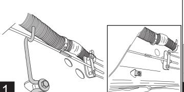
Front Idler Linkage: Thread supplied bolt (10) in about half way into the first sheetmetal tab / hole from front. Set linkage over bolt and Tighten lower bolt (10) to 16ft-lbs (22N m). Finger tighten nut (11) onto bolt (10). Install bolt (12) and torque to 16 ft-lb (22N m). Next torque lower nut (11) to 16 ft-lb (22N m) using wrench to hold lower bolt in place.
