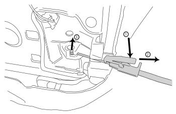
Route trigger wire into the door. Poke hole through rubber grommet and push wire through. Pull back door weather guard and run wire across rear door panel to door switch plug.
