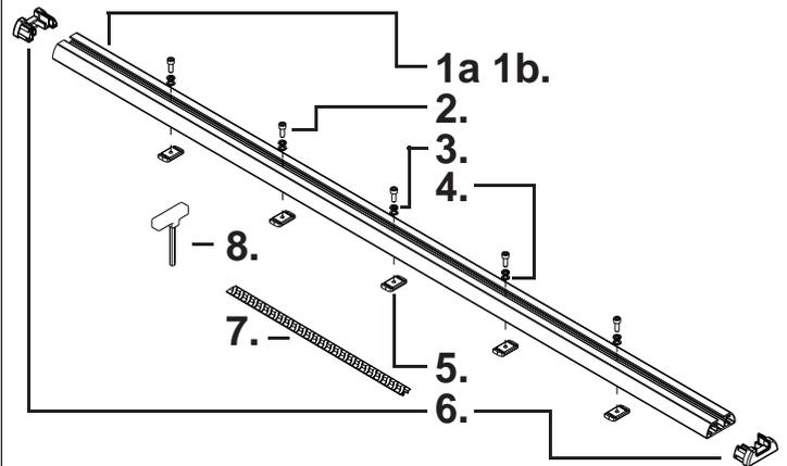
**1** Install all security screws using spring washers, flat washers and channel nuts. Finger tighten.
