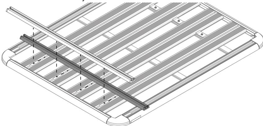
**3** Make sure the channel nut is located across the plank as shown.
