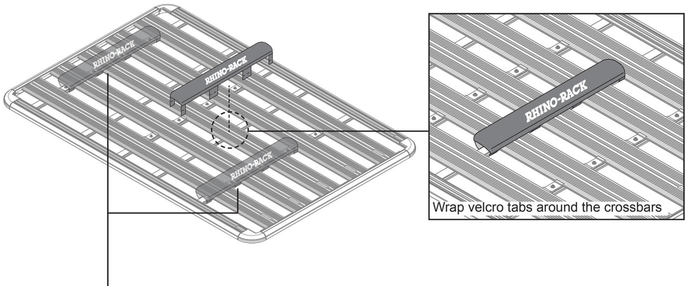
Note: Pioneer Wrap Pads Can be fixed in any position (across three tray planks) on the tray.
