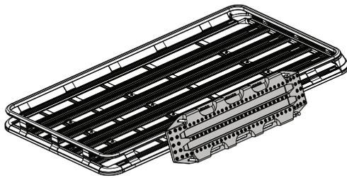
Pioneer Tray with welded sides does not require support bracket.
