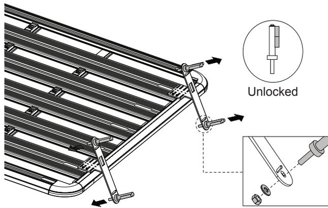
**3** Place the Maxtrax through the mounting pins, onto the brackets. Make some adjustments if required. Tighten the nuts and lock the mounting pins.
