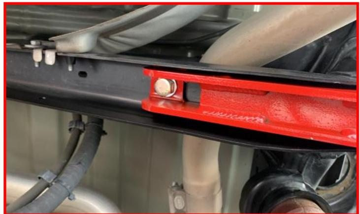
Attach the **track bar bracket support tab** to the factory track bar mount using the **track bar bracket nut plate**, the supplied **M12 x 35mm bolt and washers** and tread locker. Tighten all mounting hardware at this time.
