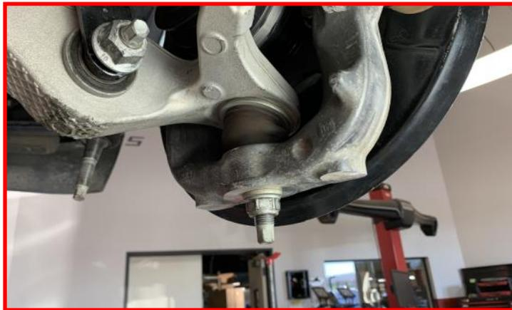
Remove **(4) sway bar mounting bolts** from the frame and retain the factory hardware. Gently hang sway bar from end links.
