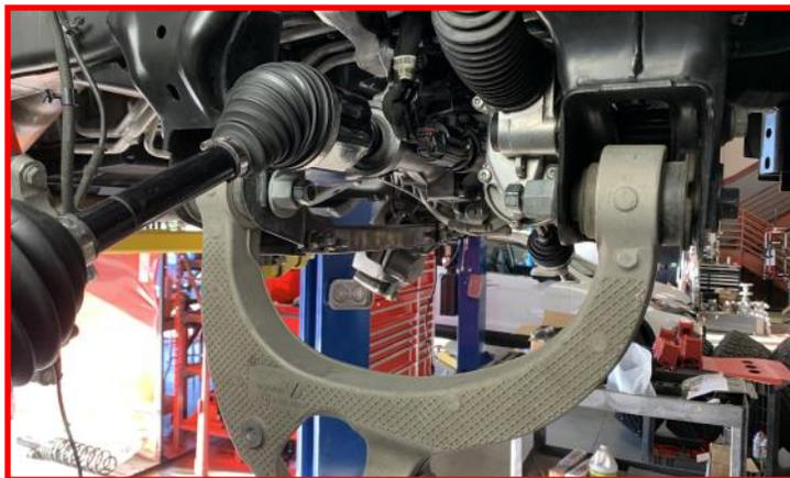
Remove the **lower control arm** from the frame. Be sure to retain factory alignment cam bolts, cams and nuts.
