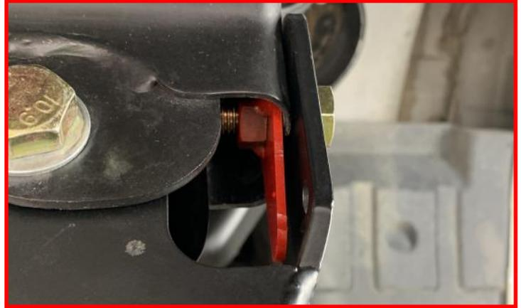
Install the track bar into the track bar bracket using the factory hardware. Do not tighten at this time.
