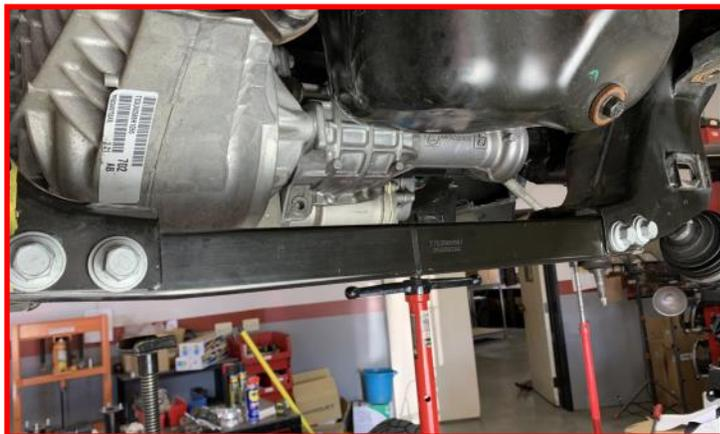
Mark the driveshaft to pinion flange location. Remove the front driveshaft hardware from the flange. Let driveline hang out of the way. Discard the factory hardware.
