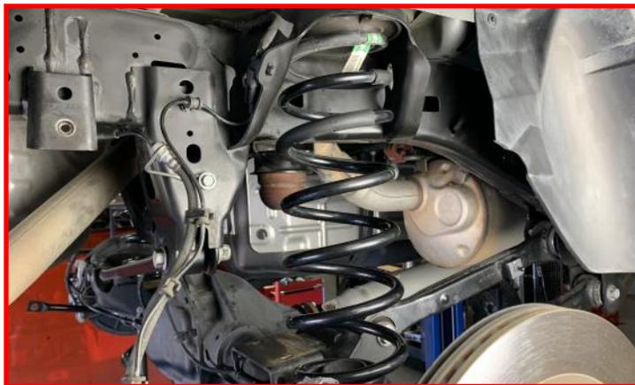
Remove both the **rear upper control arm pivot bolt** at the axle. Retain the factory mounting hardware.
