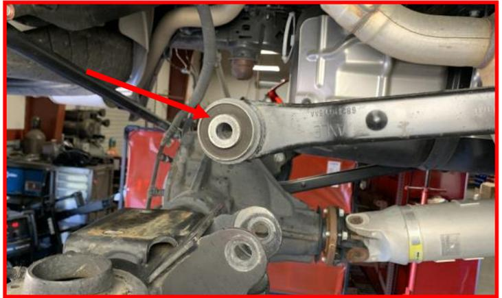
Install the supplied **passenger upper control arm bracket** to the axle using the supplied **M10 x 35mm bolts, nuts and washers**. Do not tighten at this time.
