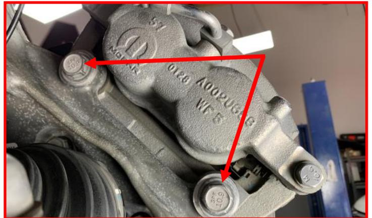
Remove **brake rotor retaining bolt** and remove the rotor. Retain the factory hardware.
