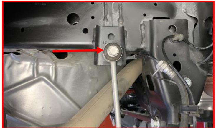
Remove the **lower sway bar end link** at the **sway bar**.
