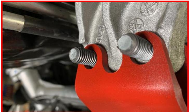
Install the **rear differential drop** onto the rear factory differential mounting point using the **using the supplied M12 x 35mm bolts, nuts and washers**.
