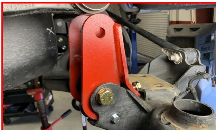
Install the supplied **M8 bolt, nut and washer,** through the axle mount and the upper control arm bracket. Do not tighten at this time.
