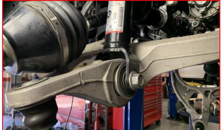
Remove the **ABS wire bracket** on the inside of the knuckle.
