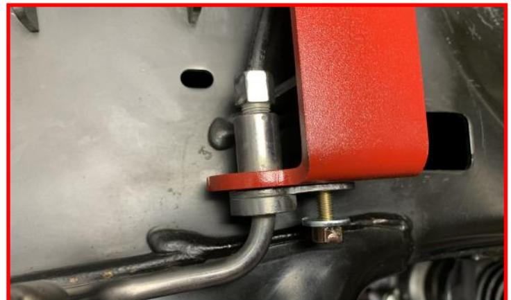
Using the factory brake line mounting hardware, install the **brake line drop bracket** onto the factory brake line mounting location.
