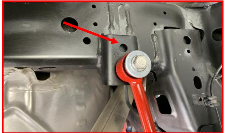
Install the completed **sway bar end link assembly** onto the sway bar using the supplied **M12 x 70mm bolt, nut, flat washer** and **fender washer**. Do not tighten at this time.
