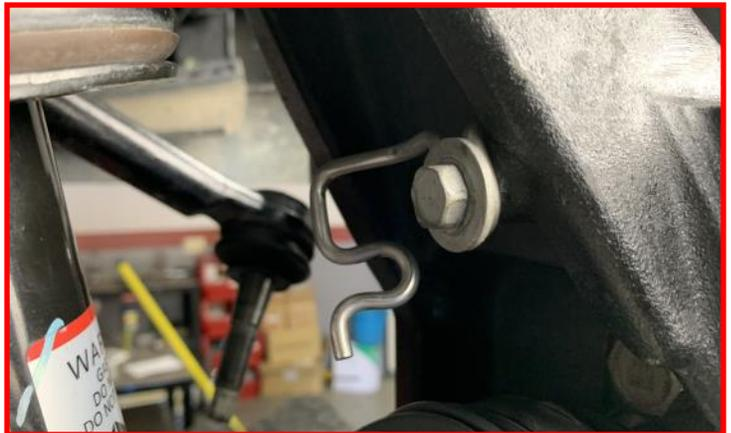
Remove the **ABS wire harness retaining clips** that are attached the frame rail. This will allow additional length that is required to install the ABS sensor into the knuckle.
