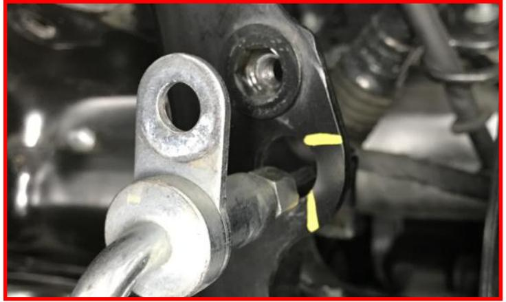
Remove brake line from factory mounting area.
