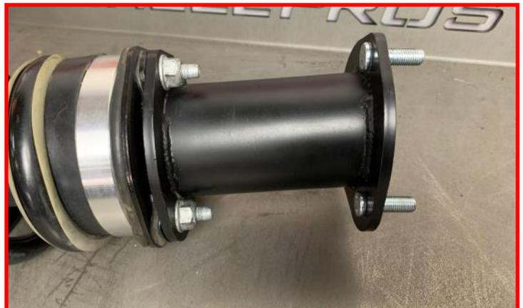
Mark the factory brake line bracket on the upper strut mount as shown.
