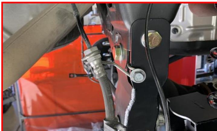
Install the ABS retaining clip into the **factory brake line bracket** location.
