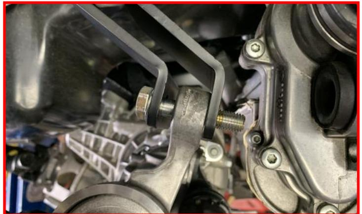
Install **shift solenoid harness bracket** onto the **(2) M12 bolts** used to mount the passenger side differential in the previous step. Install the supplied **M12 locking nuts and washers**.
