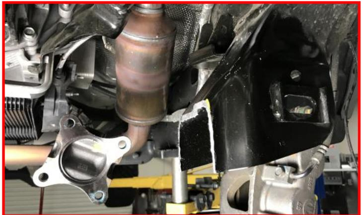
Install the **driver side differential drops** onto factory differential mounting point using the **factory bolts**. Do not tighten at this time.
