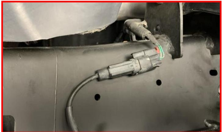
Route the ABS wire between the knuckle and the strut. Ensure the ABS wire is routed over the CV axle as well.
