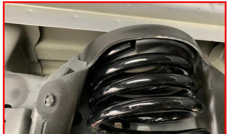
**Note: Orientate the coil so the final coil terminates at 9 o'clock on the axle side.**
