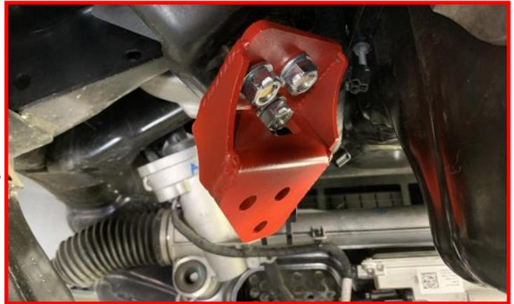
Install the **(3) factory mounting bolts** through the rear differential drop bracket and into the differential.
