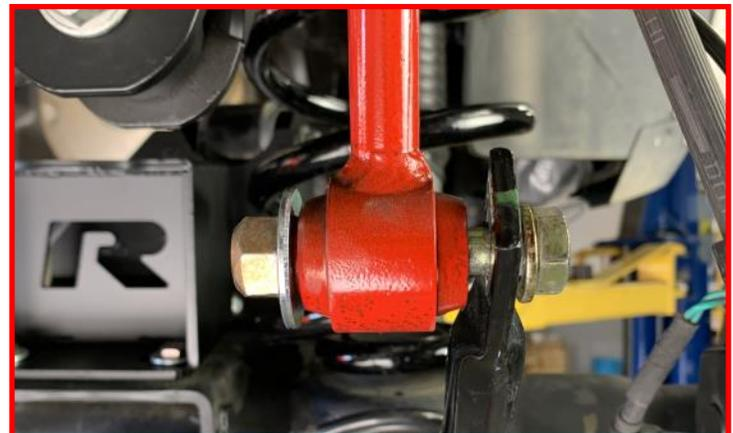
**Note:** Ensure the fender washer is installed on the bushing side.
