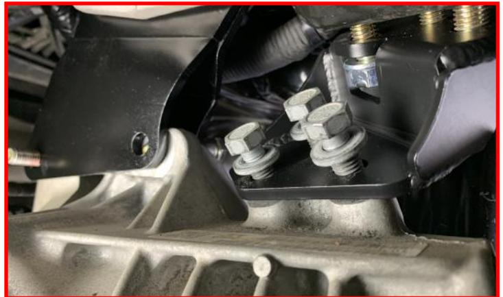
Install the provided **M12 x 60mm bolt and washers** through the **passenger side rear differential drop bracket**, the **differential housing**, then the **passenger side front differential drop bracket**.
