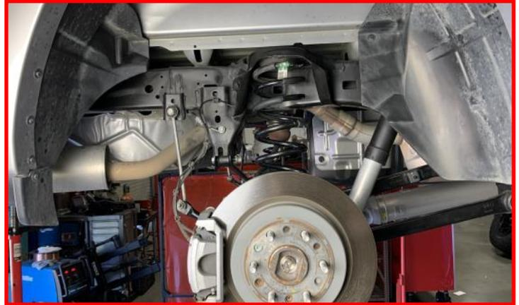
Remove the **upper sway bar end link** at the frame rail.
