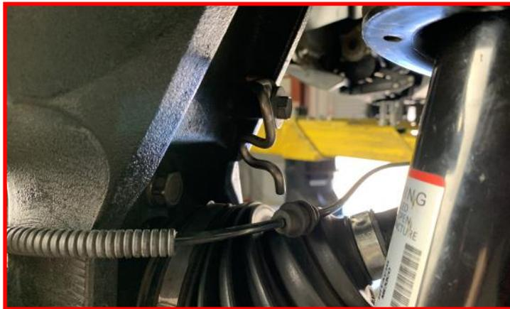
Install **ABS sensor** into knuckle using the **factory hardware**.
