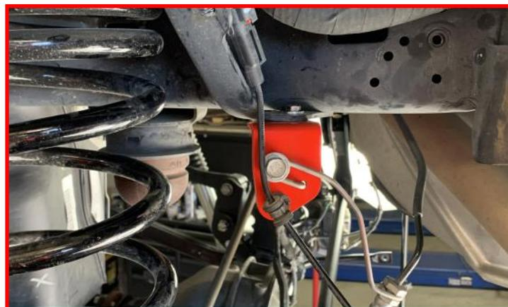
While gently pulling down on the brake line install the factory brake line bracket onto the **rear track bar bracket** using the factory hardware and supplied **M8 nut and washer**.
