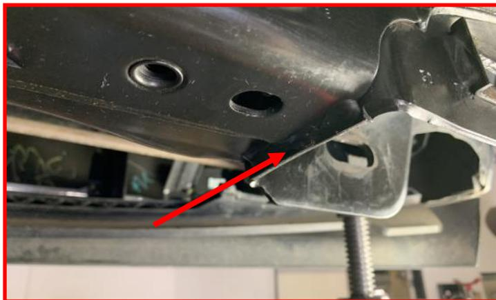
Install **front crossmember** using the supplied **cam block off plates, M18 bolts, washers, and nuts.**
