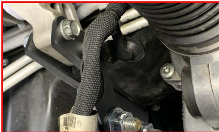
**Note:** Due the fact that there are minor differences in frame production, it may be necessary to trim the bottom edge of the front control arm pivot pocket.
