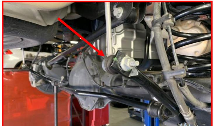
Locate and remove the **passenger brake line bracket** mounted on the frame rail.
