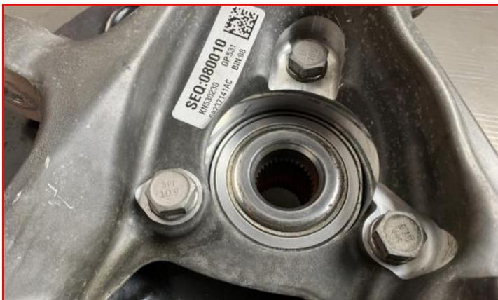
Remove hub assembly from factory knuckle.
