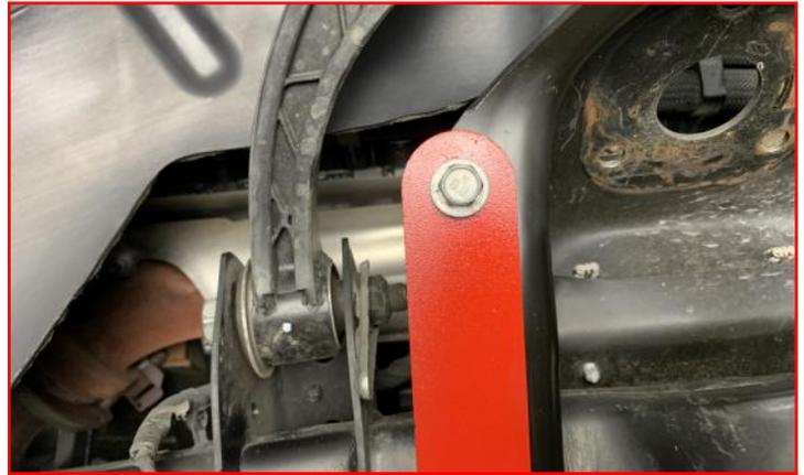
Install the completed strut assembly using the supplied M10 serrated flange nut.
