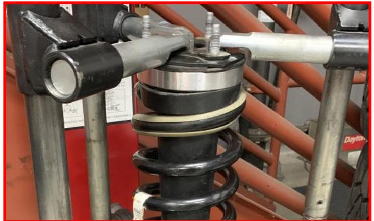
Locate the top strut extension and install using the **factory hardware.**
