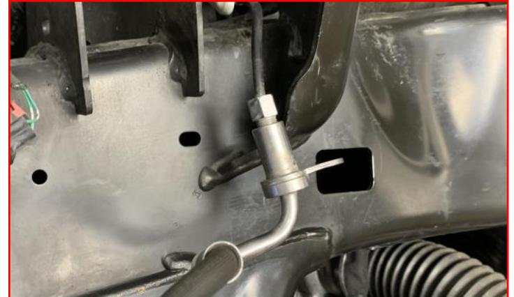
Install the **brake line drop bracket** onto the factory brake line bulkhead fitting using the supplied **M6 bolt, locking nut and washers**.
