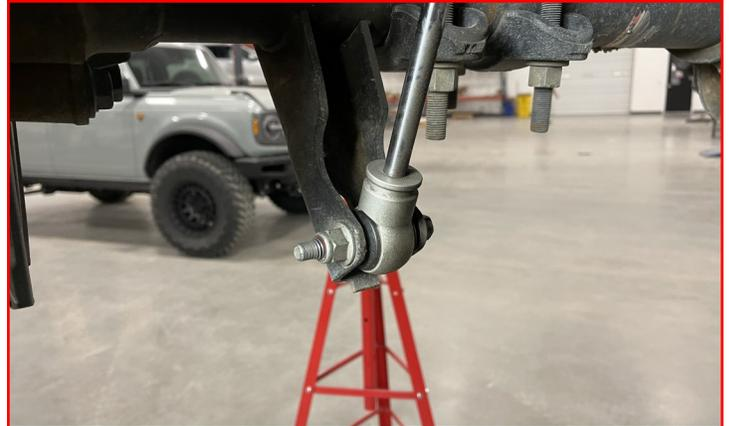
Prior to installing wheels, complete all installation steps on the opposite side. Install the wheels and lower the vehicle to the ground. Torque the lug nuts to the wheel manufacturers specs. Jounce the vehicle to settle the suspension to the new ride height. Torque the lower control arm hardware to **200 ft-lbs**, u-bolts to **110-ft/lbs** and all shock hardware to **75-ft/lbs**.
