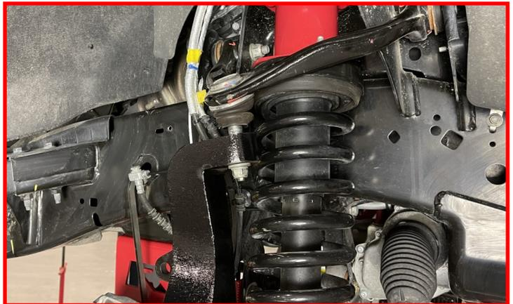
With the knuckle in place install the EIWE actuator onto knuckle using **factory hardware**.
