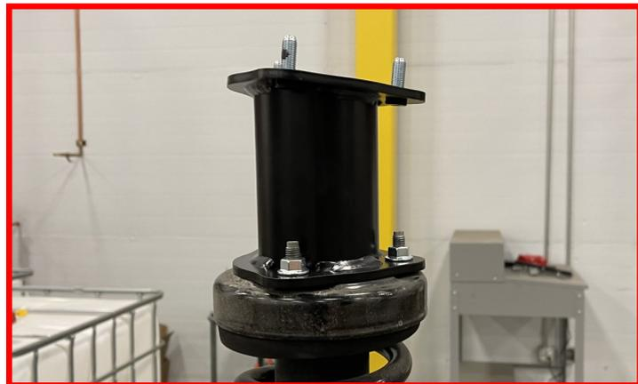
Install the completed strut assembly into the vehicle frame and lower control arms using supplied **10mm x 1.25 flange nuts and factory lower hardware**.
