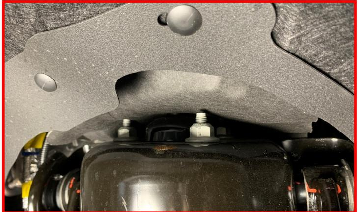
Remove the **lower strut nuts**.
