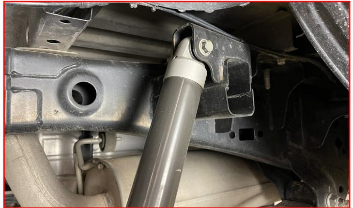
Install the rear shock into the factory axle mounting location using the factory hardware.
