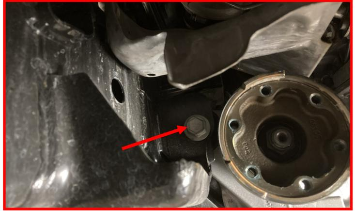
Remove the **passenger side diff mounting bolt**.
