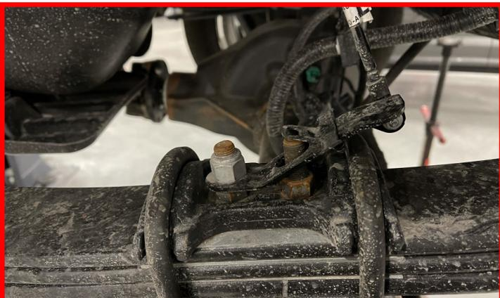
Install the rear brake line drop bracket to the frame using **factory hardware**.
