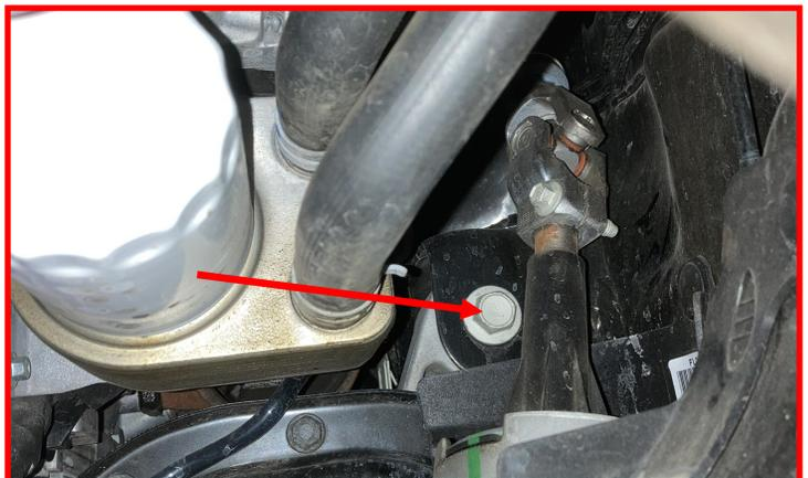
Remove the **rear diff mounting bolt**.
