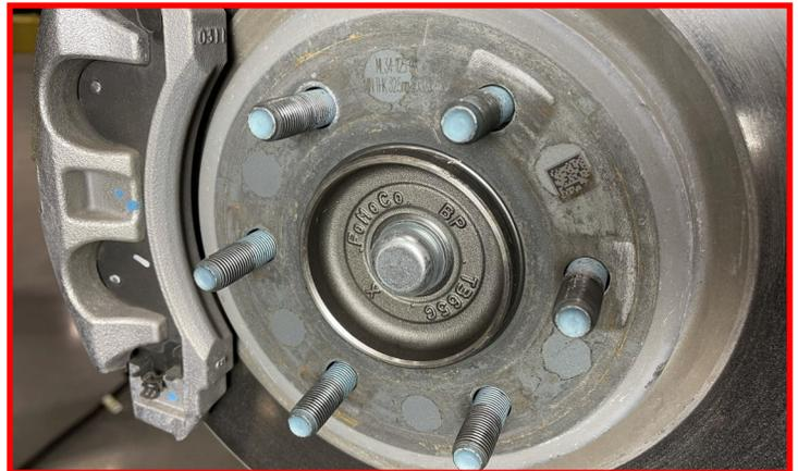
Remove the brake caliper mounting bolts from brake caliper.
