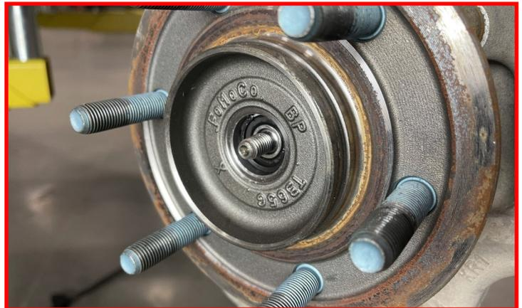
Remove the (4) bolts that attach the EIWE to the knuckle and pull both axle and the EIWE out of the factory knuckle.
