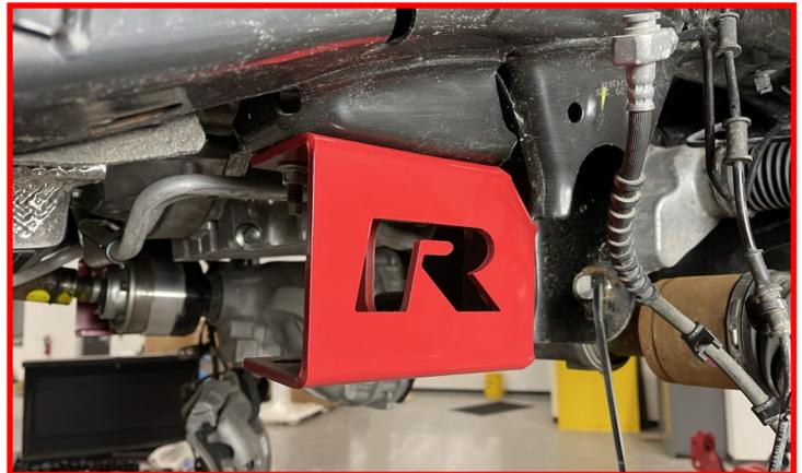
Install the **rear cross member** into the factory control arm frame pockets using **M18 x 150mm bolts, flat washers, and lock nuts**.
