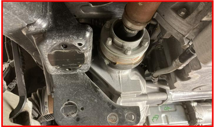
Remove the passenger side CV by striking the shaft with a hammer to dislodge it from the splines.
