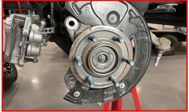
Next, remove the (3) dust shield mounting bolts and dust shield.
