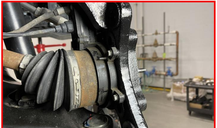
Carefully install the hub assembly over the axle shaft and into the knuckle bore. Make sure the ABS wire is located at the top of the hub.
