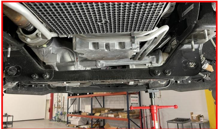
Mark the driveshaft to pinion flange location. Remove the (6) **drive shaft mounting bolts** and disconnect the drive shaft from the differential. Allow the drive shaft to rest out of the way.
