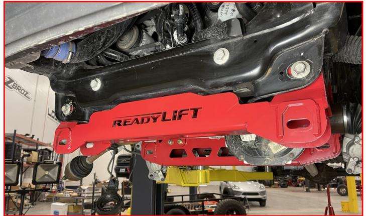
Install driver and passenger side lower control arms into the cross members using the supplied **M18 x 150mm cam bolt, eccentric plates and lock nut.**
