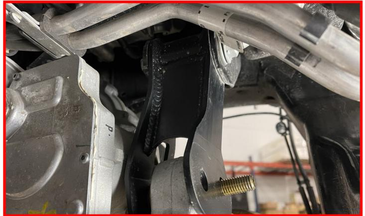
Install the **sway bar brackets** to frame using the factory hardware.
