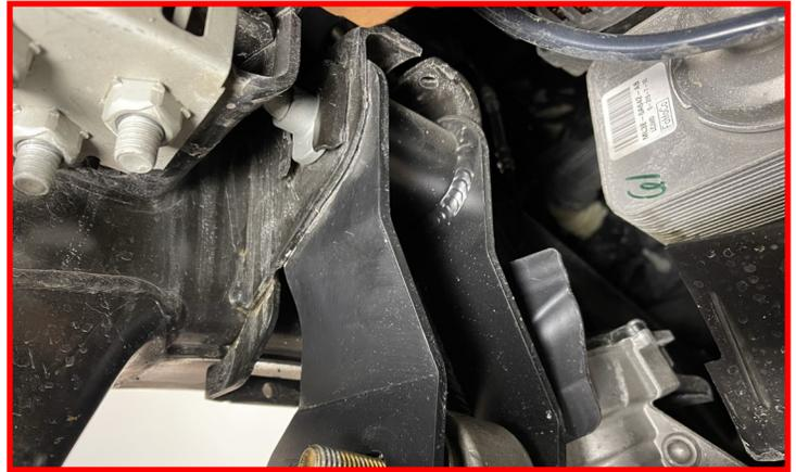
With the differential in place, install the factory **bolt and nut** through the **factory passenger side differential mount and the passenger diff drop bracket**.
