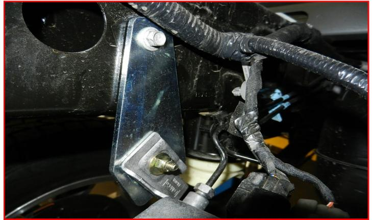
Install the provided rear shock into the factory frame mounting location using the factory hardware.
