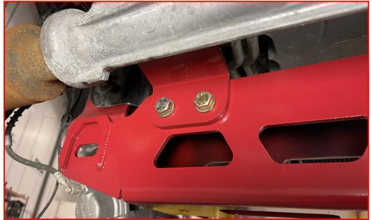
Install the **front cross member** using the **factory hardware** from the front of the vehicle facing rearward.
