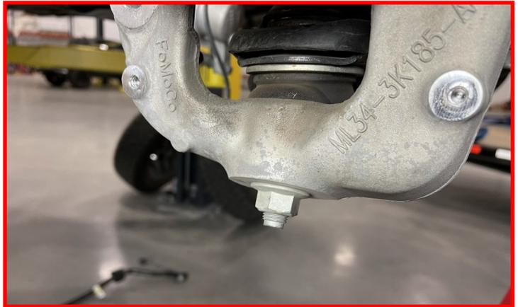
Remove the lower control arm pivot bolts.
