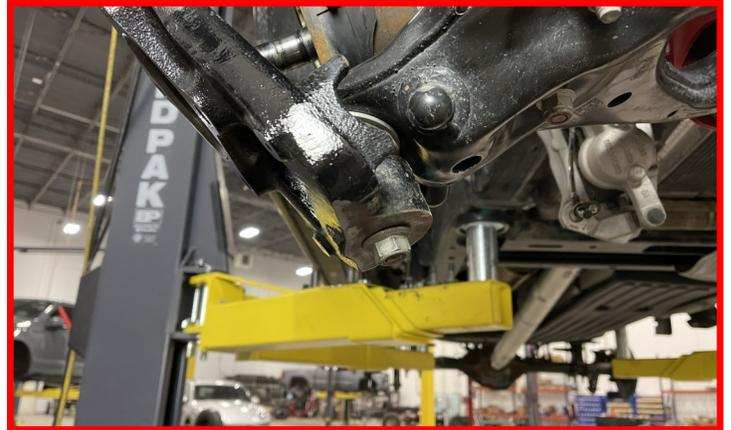
Install upper ball joint to knuckle using **factory hardware**.
