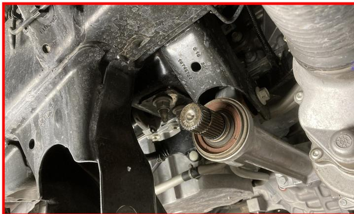
Install the EIWE onto the CV shaft. Ensure the gears are lined up and engaged properly.
