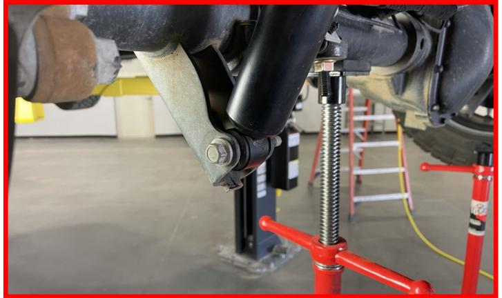
Remove the rear sensor bracket from the forward axle center pin.
