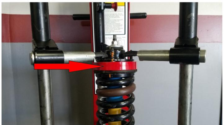
Add the strut spacer to the strut assembly making sure the alignment notches on the spacer face to the outside of the wheel well when installed on the vehicle. Use factory hardware torque **35 ft-lbs**
