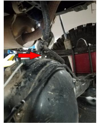
Install the ReadyLIFT parking brake extensions to the original brake line location, on the rear leaf spring use the factory hardware torque to **15 ft-lbs.** Gently reposition the brake line to the extension, fasten the brake line bracket to the extension using the provided hardware.
