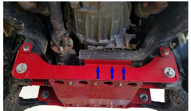
Install the ReadyLIFT skid plate. Use provided hardware, torque to **75 ft-lbs.**
