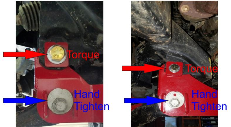
Tighten and torque the passenger differential bolts 75 ft-lbs.
