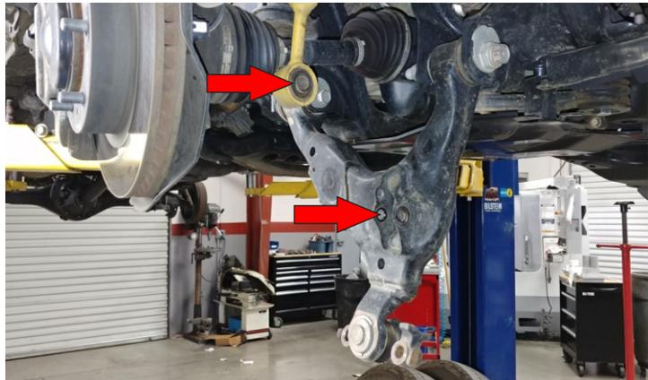
Protect the axle and ball joint boots with a wet rag or other suitable protection from grinding and welding sparks. Clean/grind off the paint/rust on the steering stop on the ball joint cradle. Weld the turn stop extension plates on their corresponding sides (match the contours of the stops) across the top and bottom.
