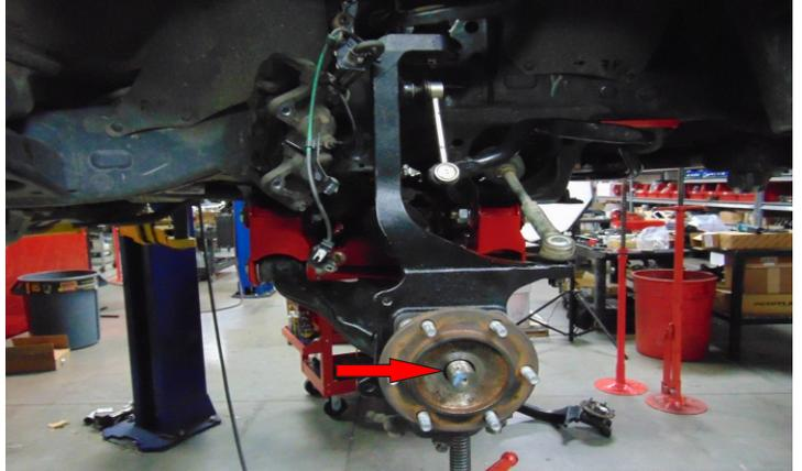
Install the **sway bar end links** to the ReadyLift knuckle. Using a 5mm allen wrench thread the stud through the knuckle. Torque to **50 ft-lbs** the nuts from the OEM knuckle can be discarded.
