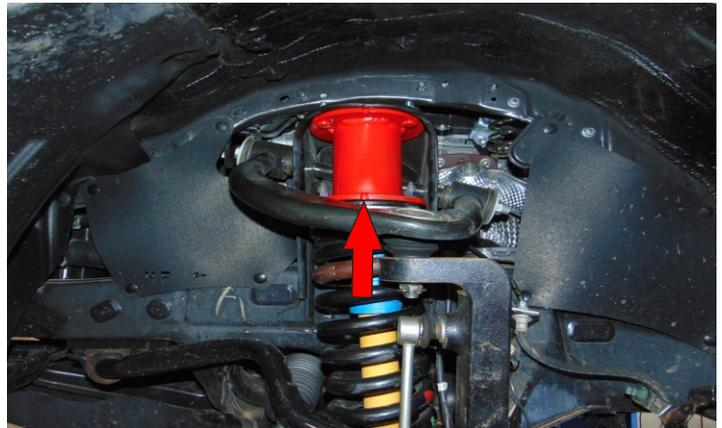
Raise the lower control arm and fasten to the **lower strut**, use factory hardware hand tight only.
