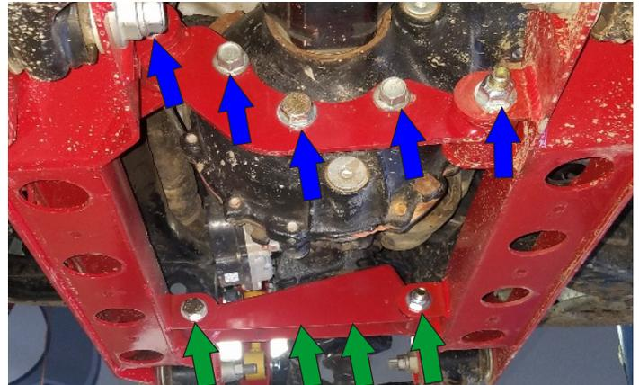
Use a 5/16 or one size larger drill bit to drill out the OEM rear crossmember use the ReadyLIFT crossmember as a guide. Install the nut plate, and fasten the two crossmembers together. Use provided hardware torque to 65 ft-lbs.
