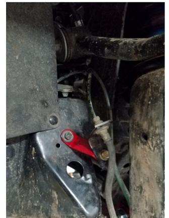
Attach the OEM ABS wire bracket to the ReadyLIFT steering bracket use factory hardware torque **10ft-lbs**. Install the wheel speed sensor to the ReadyLIFT steering knuckle. Use the factory hardware torque **5 ft-lbs**. Adjust the ABS wire as necessary, attach the ABS wire to the bracket use the factory clip.
