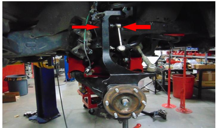
Rotate the tie rod end 180 degree, and attach to the ReadyLIFT steering knuckles. Torque to 60 ft-lbs, then tighten until the castle nut aligns with the cotter pin hole, install cotter pin.
