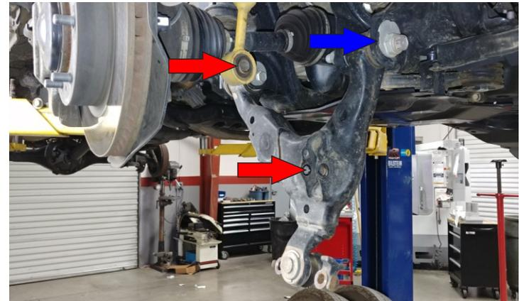
Remove the LCA from the vehicle. Loosen but do not remove the upper control arm. Hold onto the strut, remove the upper strut hardware, remove the strut from the vehicle.
