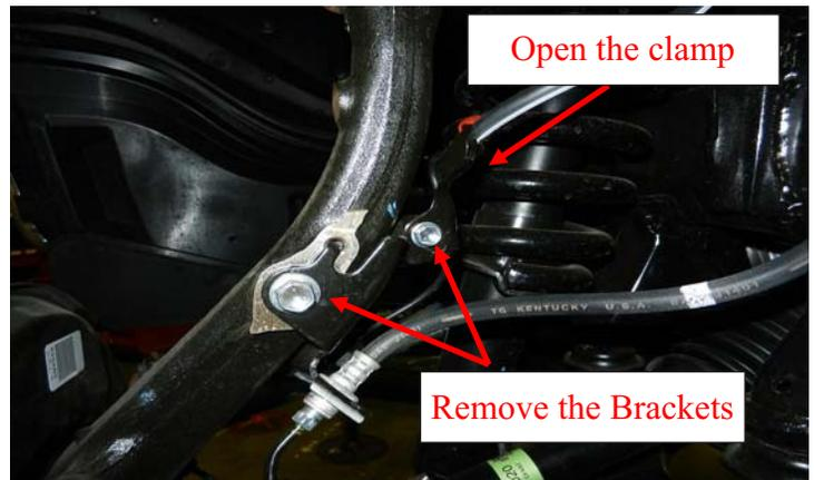
Remove the wheel speed sensor from the steering knuckle.
