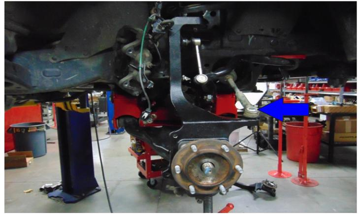
Tighten and torque the front and rear crossmember.
