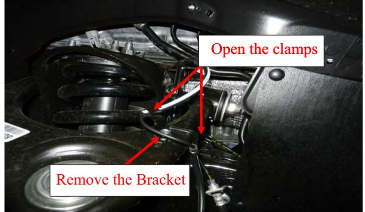
Remove the brake line from the frame and steering knuckle.
