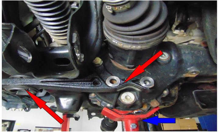
Install the new ReadyLift crossmembers using provided hardware, and cam block off plates. The cam block off plates have **notches cut**, start with the notches up you, can turn them 90 degrees for different fitments for frame deflection. Do not tighten hardware at this time.
