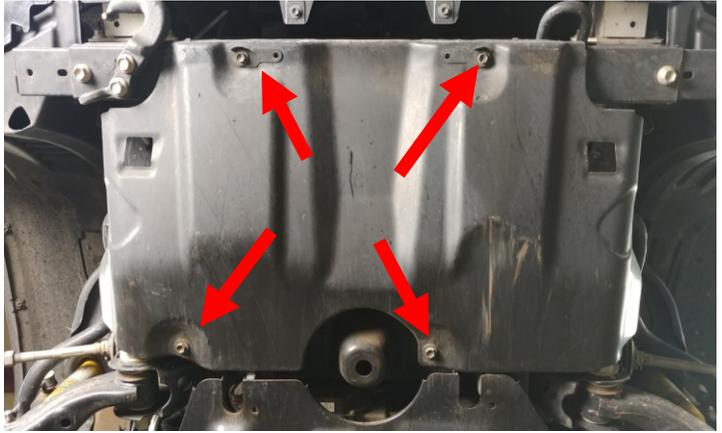
Remove the differential gravel guard.
