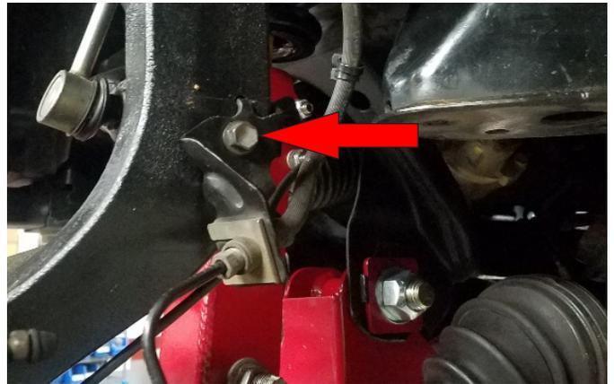
Install the ReadyLIFT front brake line extensions to the original brake line location on the frame using the factory hardware. Gently reposition the metal brake line to the extension fasten the brake line bracket to the extension using the provided hardware.
