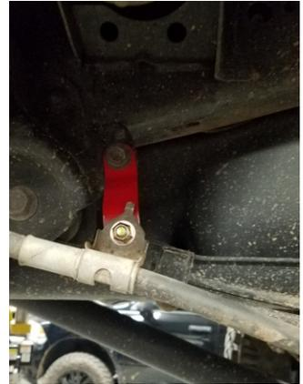
Parking brake clarification: The straight/flat bracket attaches near the spring perch toward the front of the spring. The Z shaped bracket mounts closer to the tire/mid spring.
