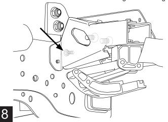
Next, re-insert nut on left side of bracket, bring forward stud by tightening until flushed with sheet metal.
