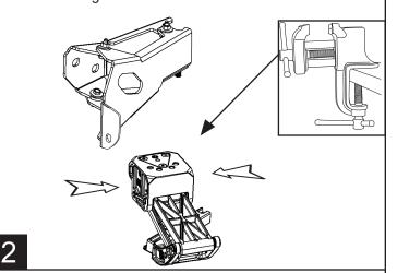
Attach bracket assembly to linkage as shown below.
