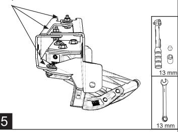
Push the two studs on the left side back enough to only expose about 1/4 of the stud. Remove Bracket and discard or store away.
