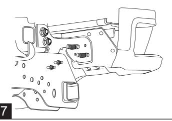
Re-insert nuts on right side using a 6" extender on wrench to reach studs. Tighten both nuts, making sure bracket remains flush and square.
