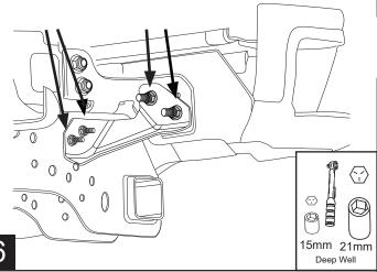
Add nut back to the stud on top right side (see arrow) of the 2 left studs, that stud won't be needed.
