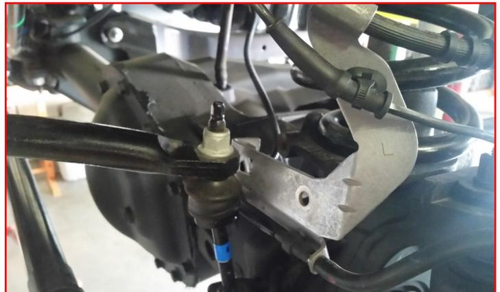
Support the axle with a suitable jack and remove the lower shock hardware from the axle mount. Retain factory hardware.
