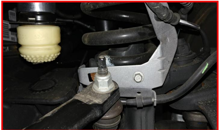
Install the supplied brake line bracket to the factory brake line using **5/16" bolts, washers, and nuts**. Install the bolt facing outwards. Torque to **10 ft-lbs**. Gently pull the metal brake line down while lining up the brake line bracket to the original holes in the frame. Install using **factory hardware**. Torque to **5 ft-lbs**.
