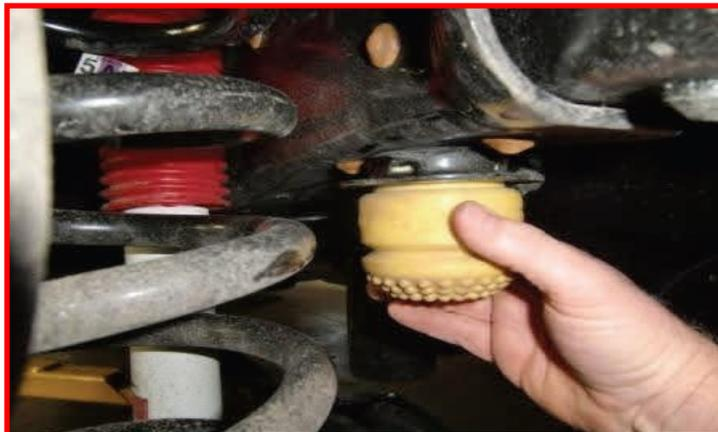
Mark a line parallel to the frame across the edge of the outer lip of the bump stop mount.
