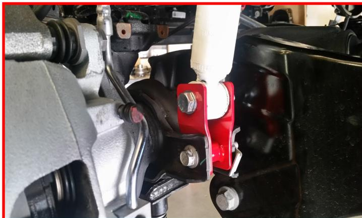
Remove stock rear shocks and install aftermarket rear shocks that are provided in this kit. Do not tighten hardware at this time.
