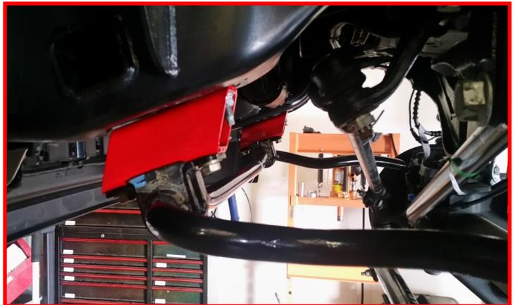
Attach the factory brake line bracket at the axle using **factory hardware**.
