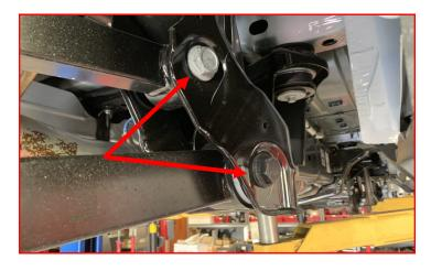
Lower the axle just enough to remove the springs.
