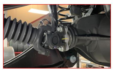
Rotate the axle to release radius arms from the mounting location.
