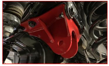
Install track bar using factory hardware. Do not tighten at this time.
