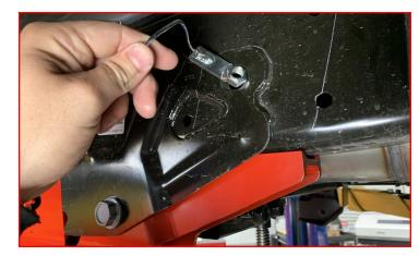
Tighten 1/2" bolts first, Ensure the drop bracket is resting flush against the frame rail and torque to 80 ft-lbs.
