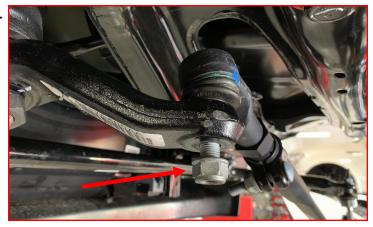
Remove the pitman arm nut. Using a pitman arm puller, remove the pitman arm from the steering box sector shaft.
