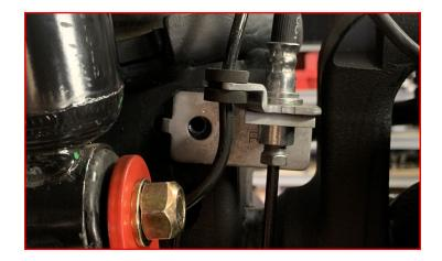
Install the front wheels. Lower the vehicle to the ground. Torque the lug nuts to the wheel manufacturers specs. Torque the lower shock hardware to 90 ft-lbs., the radius arms and track bar hardware to 200 ft-lbs.
