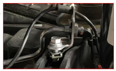
Install the ABS bracket to the axle using factory hardware.
