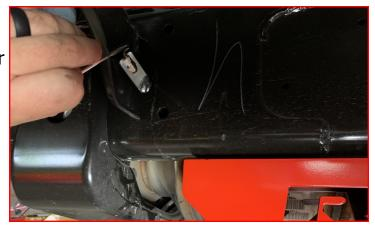
Once lined up with the lower mounting holes, install the 1/2" bolts and washers. Leave loose at this time.
