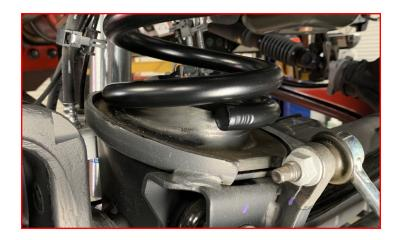
Install front shocks using factory lower hardware and provided upper hardware. Do not tighten factory hardware at this time.
