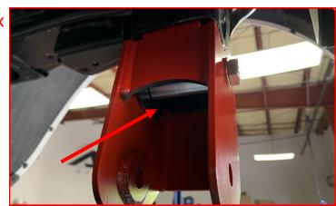
Install the 3/8" bolt, washer in the inside hole.
