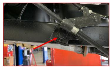
Remove brake line bracket from axle. This will allow the ABS sensor harness and brake line to have slack when lowering the axle.
