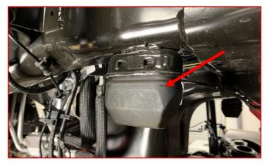
Install the supplied extended bump stops. To aid in install, lube the mounting end with a soap and water mix.
