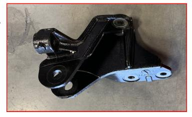
Install replacement track bar drop bracket using factory hardware and provided M14 nuts and washers.
