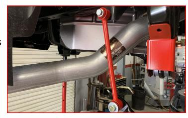
Install the sway bar end links using M12 bolts, washers, and c-lock nuts. Ensure the fender washer is installed on the outside of the bushing. Do not tighten at this time.
