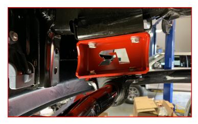
Install brake line drops to the brake line bracket using 5/16" bolts, washers and nuts . Do not tighten at this time. Attach brake line and drop bracket to the inside frame rail using the factory hardware. It will be necessary to gently pull down and bend the metal brake line on the driver side to gain the slack needed.
