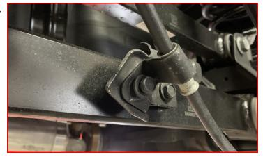
Install ABS sensor harness and brake line bracket onto axle.
