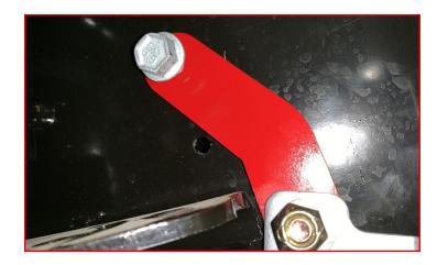
Install the ABS sensor harness and brakeline bracket to the radius arm using factory hardware.
