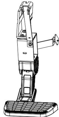
**For 6.5' bed lengths components must be configured for Passenger or Driver-side as shown.**
