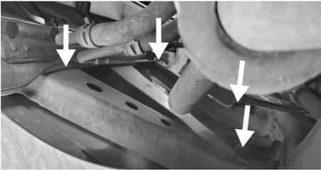
Fig. 6: Install spacers here
