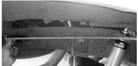
Fig. 7: Passenger side reservoir bracket location rear
