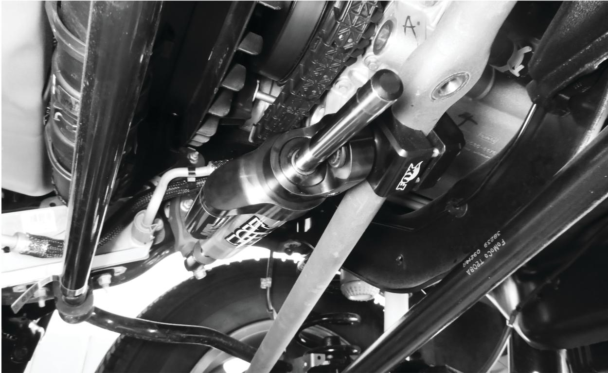
Fig. 2: Loosely clamp stabilizer to drag link.
