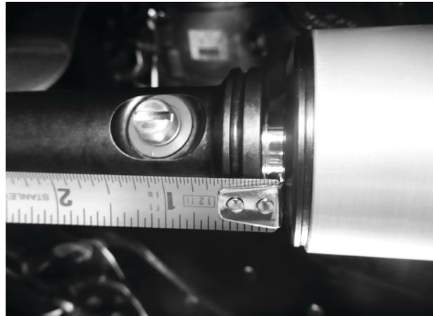
Fig. 1: Eyelet installed with 1/8" of shaft exposed.
