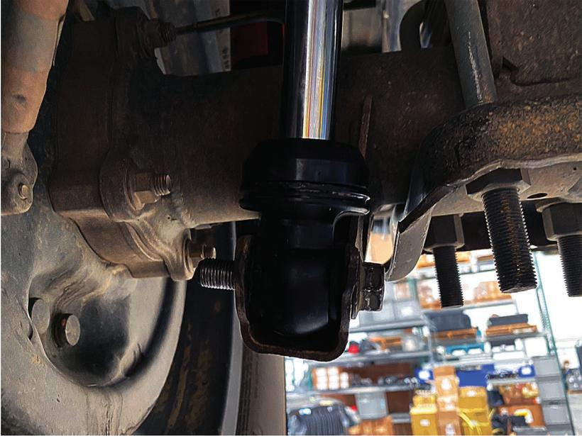
Figure 3: Rear lower eyelet installed
