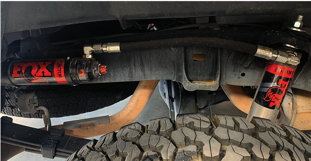
Figure 2: Passenger side shock assembly
