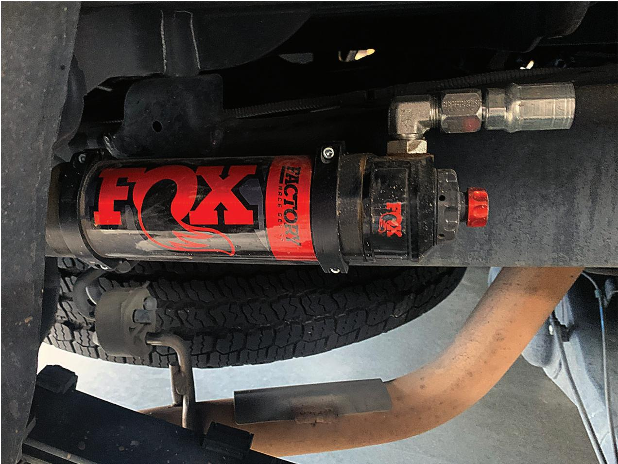
Figure 6: Installed reservoir
