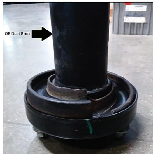
Figure 6: Top-mount and dust cover for removal
