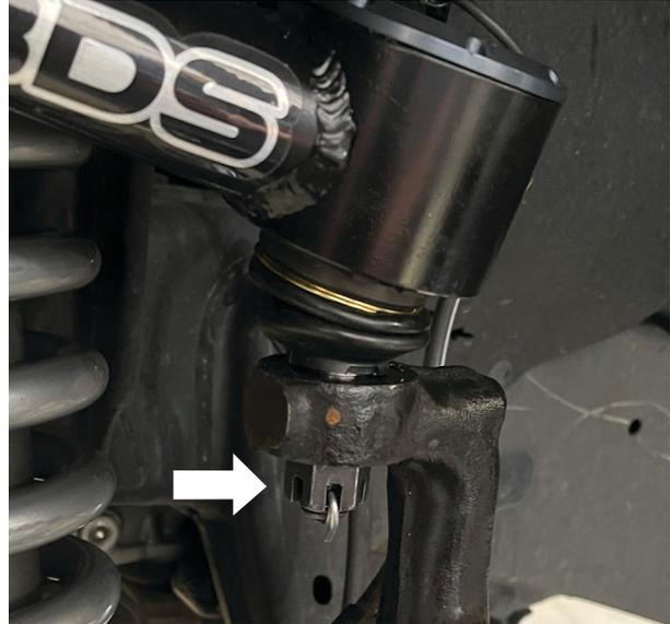
Fig. 6: Loosen upper control arm castle nut.
