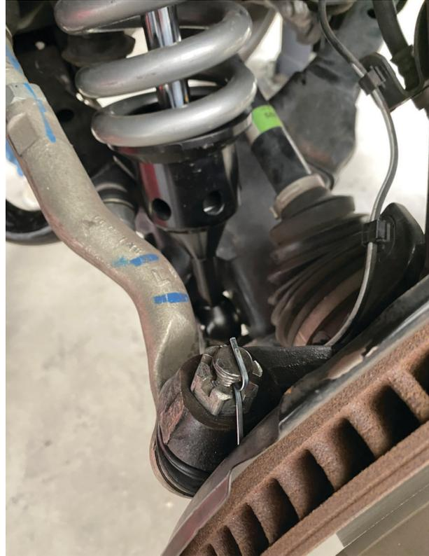
Fig. 10: Reinstall the tie rod end link.
