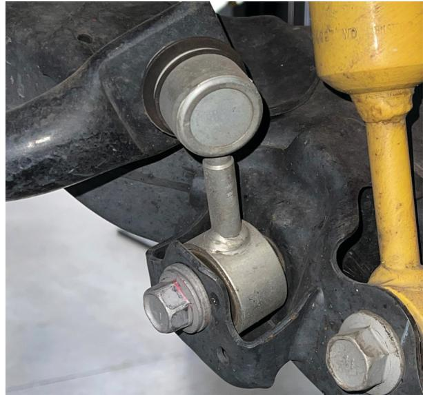
Fig. 2: Disconnect the sway bar end link.
