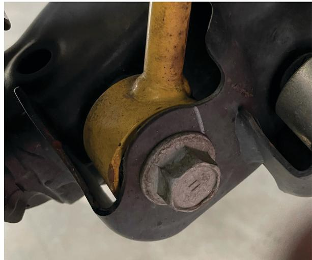
Fig. 5: Remove bolt on lower shock mount.
