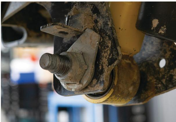
Fig. 26: Loosen the lower mounting bolt.
