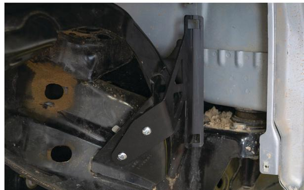
Fig. 31: Mount the reservoir bracket.
