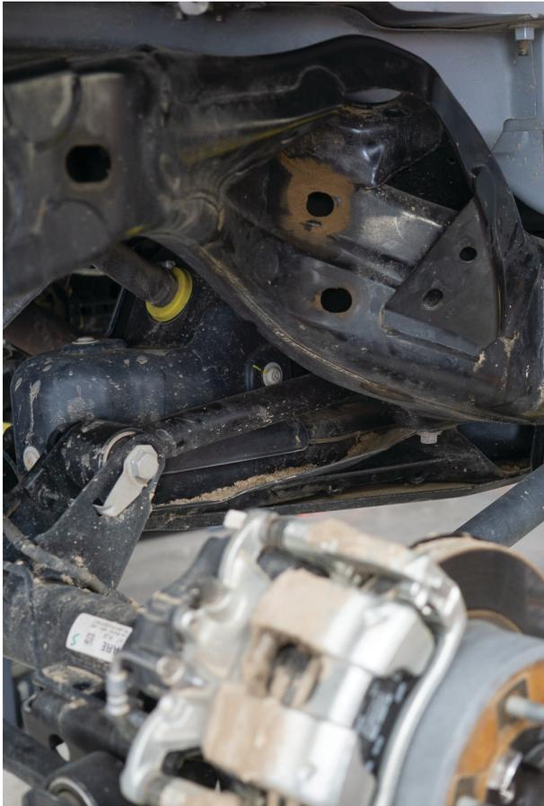
Fig. 28: Remove the stock coil-over.
