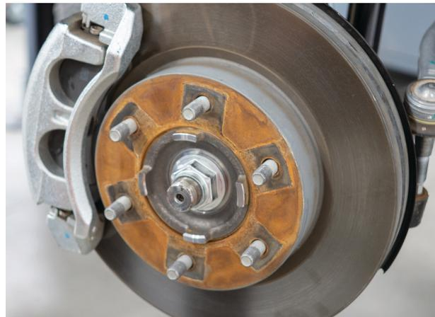
Fig. 18: Fasten the axle nut.
