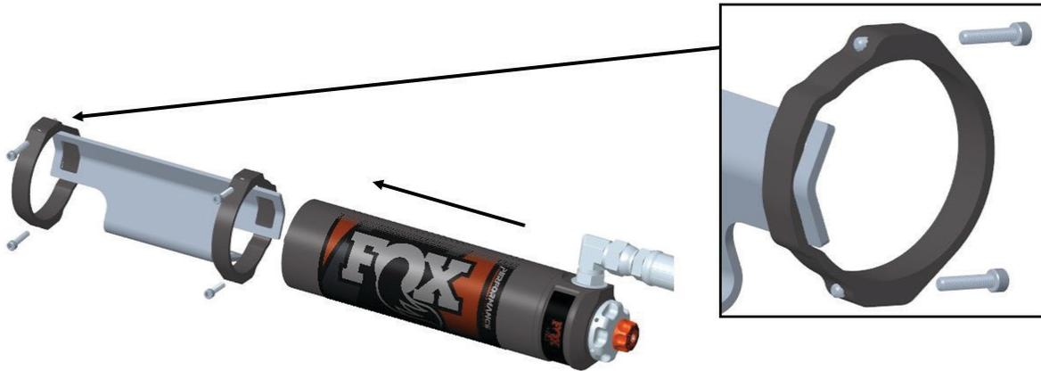
Fig. 16a: Diagram of reservoir and bracket interface.
