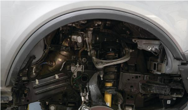
Fig. 1: Pull the fender liner.
