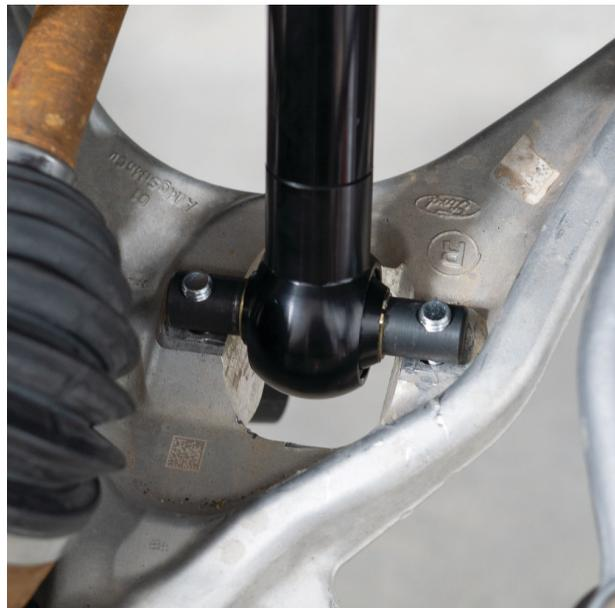
Fig. 15: Fasten the bar-pin bolts.
