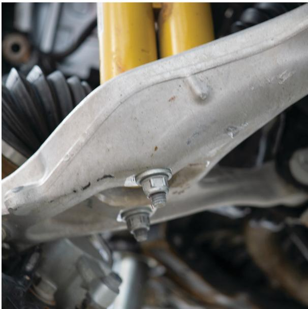
Fig. 11: Take off the bar-pin bolts.
