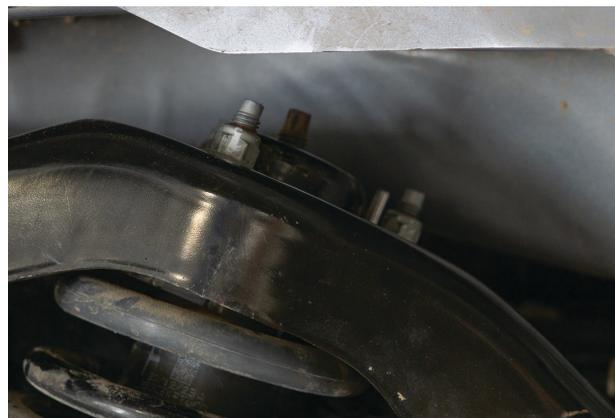
Fig. 27: Do not remove the center nut.
