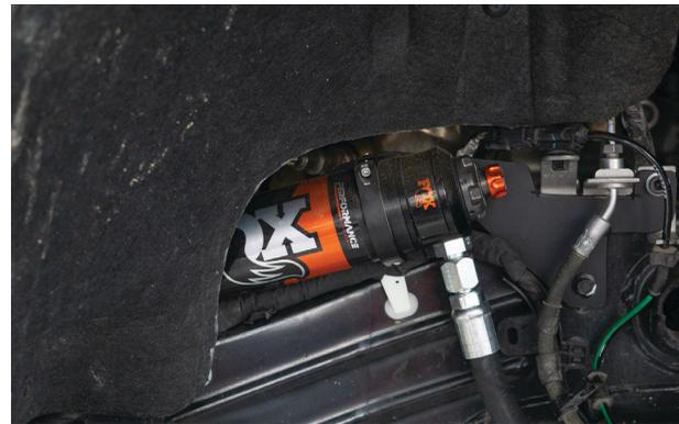
Fig. 23: Cut fender liner.
