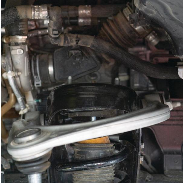
Fig. 9: DO NOT remove the center nut.
