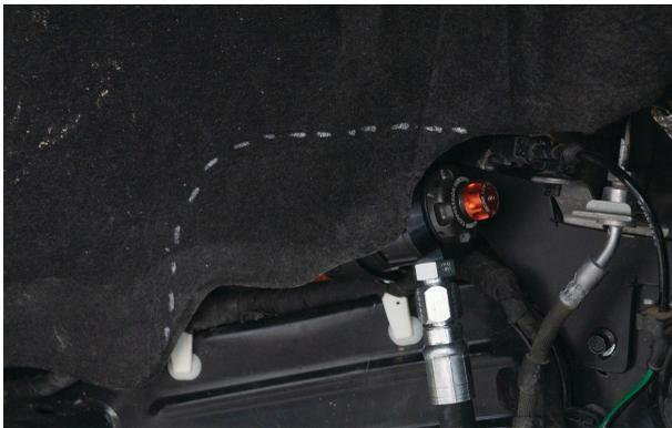
Fig. 22: Test fit the fender liner.
