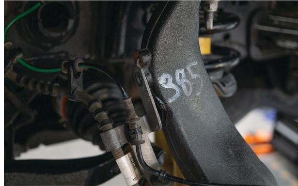
Fig. 4: Disconnect brake line bracket.
