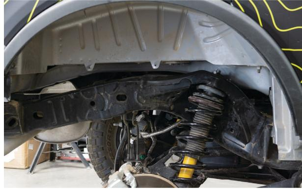
Fig. 24: Pull the fender liner.
