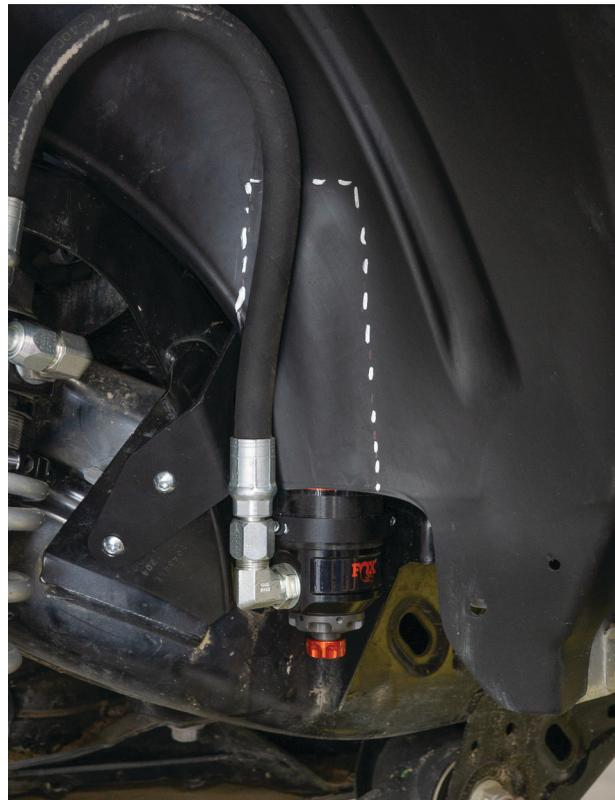
Fig. 36: Test fit the fender liner.
