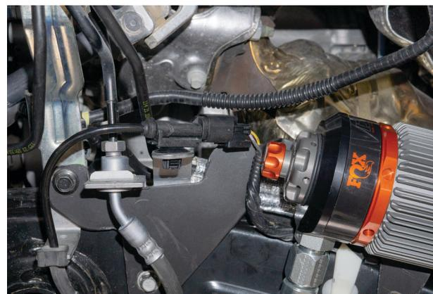
Fig. 26: Fish the ABS wire through the bracket.
