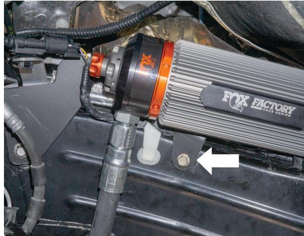
Fig. 27: Install the self-tapping screw.
