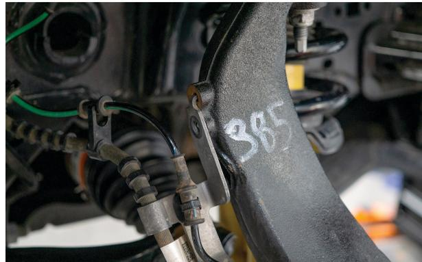
Fig. 2: Disconnect brake line bracket.
