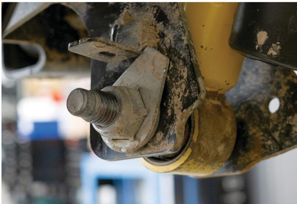
Fig. 31: Loosen the lower mounting bolt.
