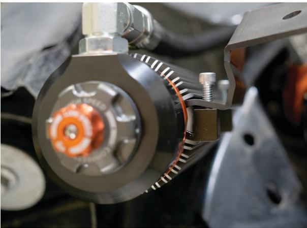
Fig. 37: Mount the reservoir bracket.
