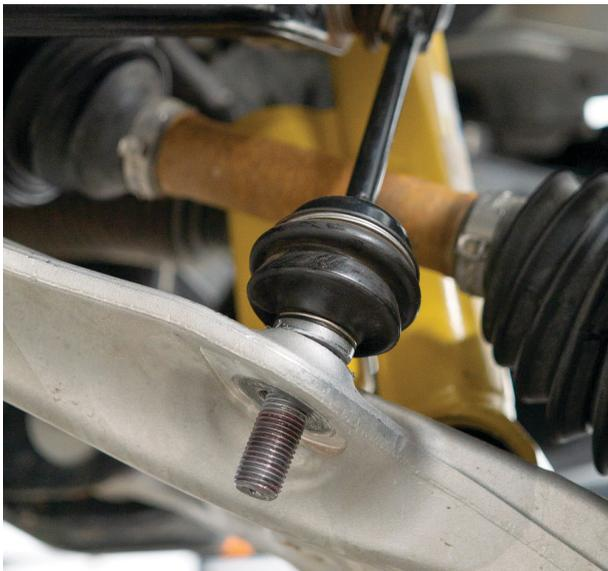
Fig. 4: Disconnect sway bar end link.
