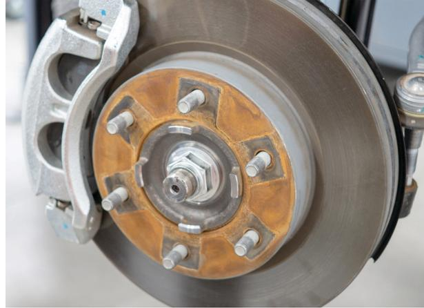
Fig. 15: Fasten the axle nut.
