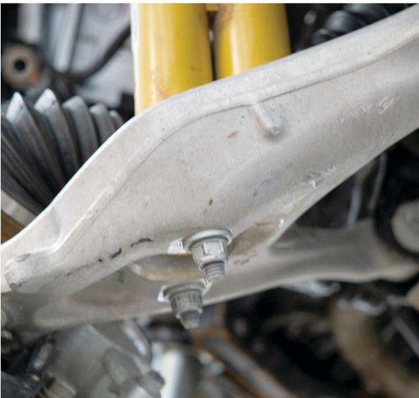
Fig. 9: Take off the bar-pin bolts.
