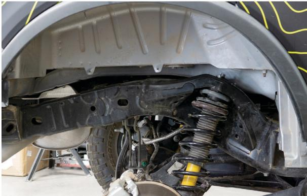
Fig. 29: Pull the fender liner.
