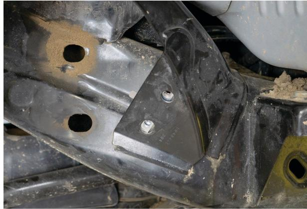
Fig. 40: Locate the backing plate's speed nuts with the holes in the frame.
