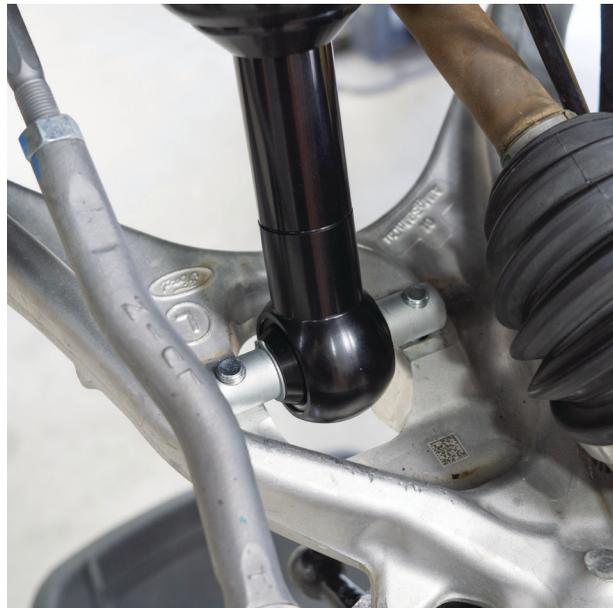
Fig. 13: Fasten the bar-pin bolts.
