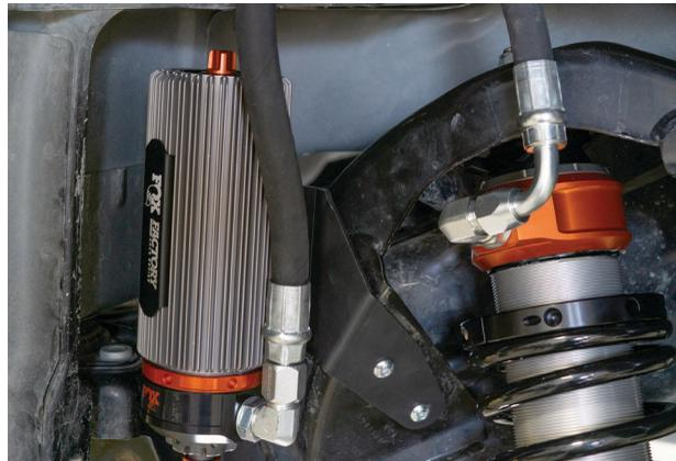
Fig. 42: Mount the reservoir bracket.
