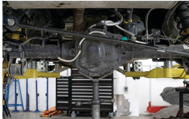
Fig. 30: Support the differential.
