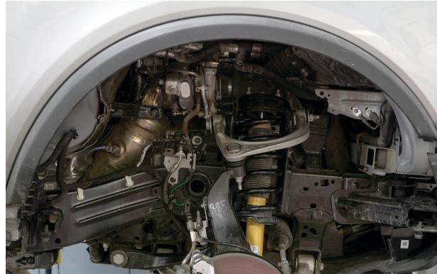
Fig. 1: Pull the fender liner.
