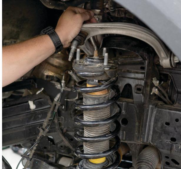
Fig. 8: Free the coil-over from the coil bucket.
