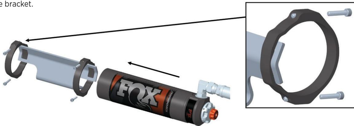
Fig. 12: Diagram of reservoir and bracket interface.
