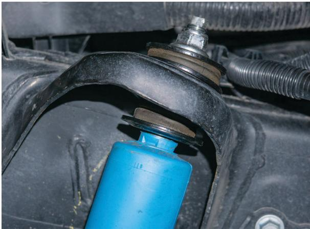
Fig. 16: Remove stem top nut.
