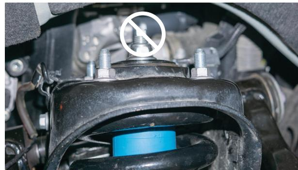
Fig. 7: Remove the four top hat nuts.
