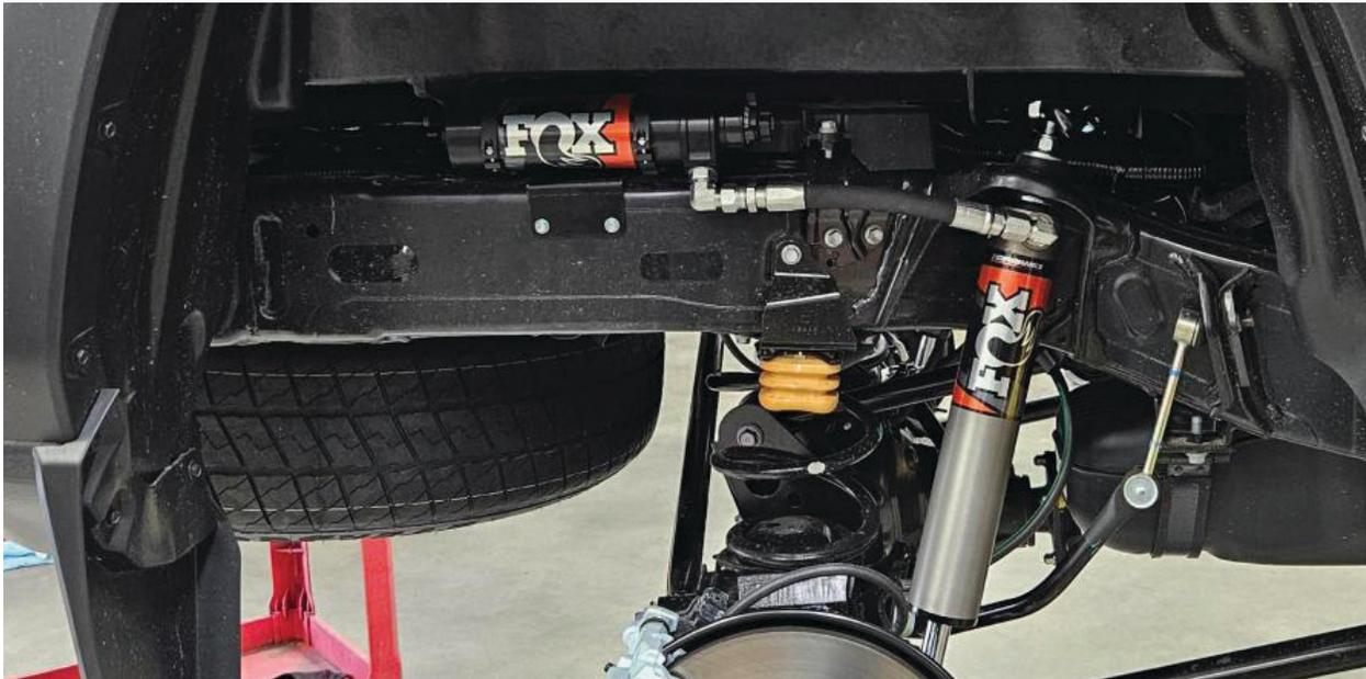
Fig. 22: Mount the reservoir to the bracket (passenger side shown).
