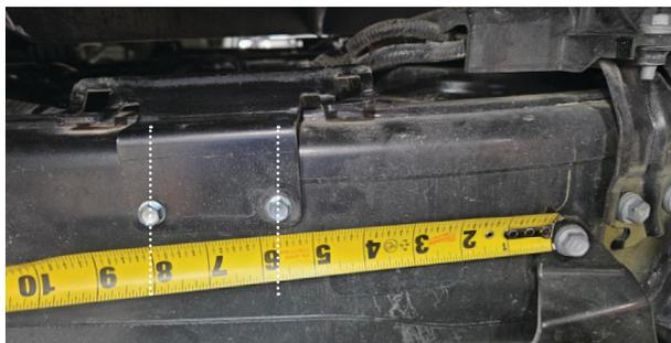
Fig. 19: Drill two pilot holes; fasten the screws.
