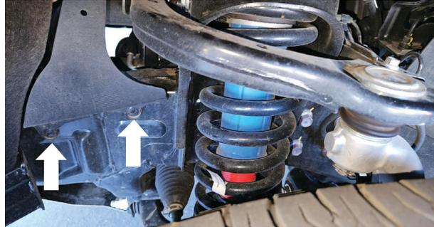
Fig. 4: Remove the plastic plugs of the splash guard.
