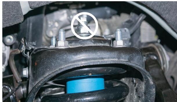
Fig. 6: Remove the four top hat nuts. Do NOT remove the center nut.
