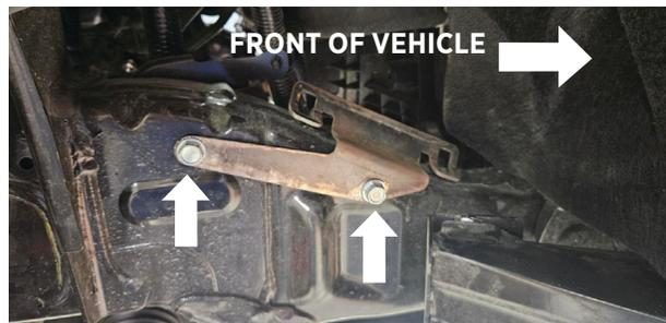
Fig. 5: Install the reservoir bracket assembly.
