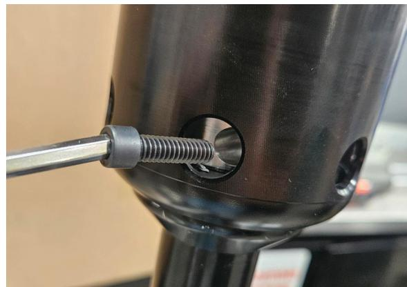
Fig. 16: Screws to clamp spacers to shaft.
