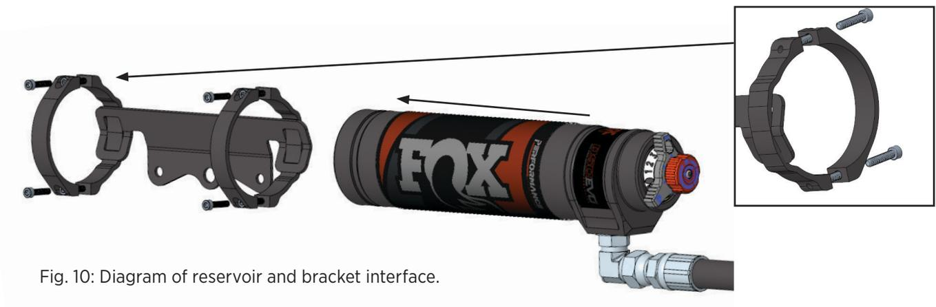
Fig. 10: Diagram of reservoir and bracket interface.
