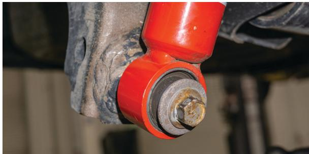
Fig. 18: Remove lower shock mount bolt.
