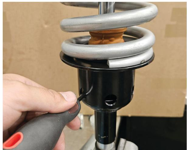
Fig. 14: Lift the bump stop with a screwdriver.
