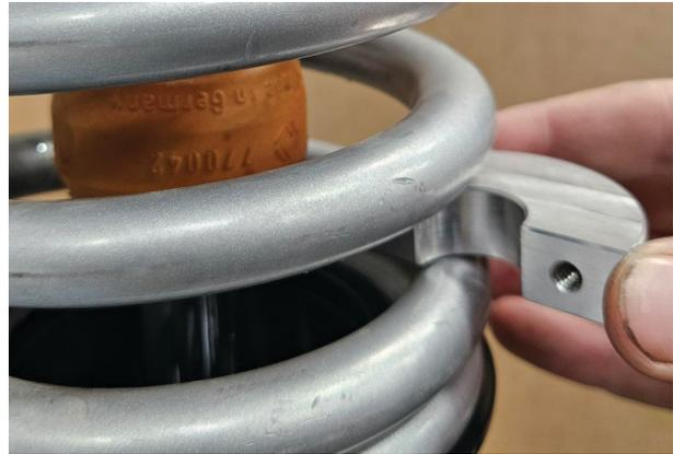
Fig. 15: Slide spacers through spring.
