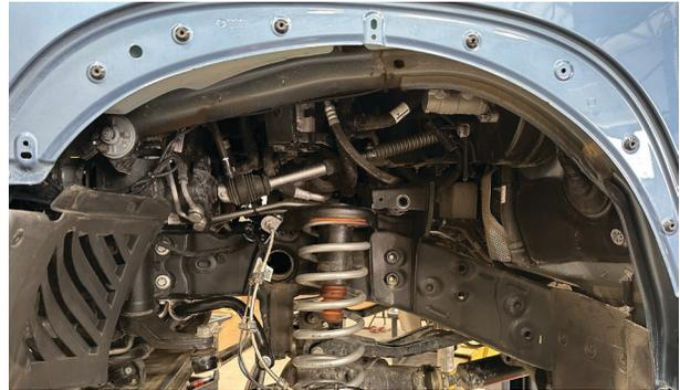
Fig. 1: Pull the fender liner.
