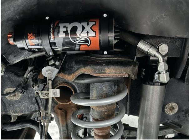
Fig. 6: Mounted Performance Elite Reservoir.
