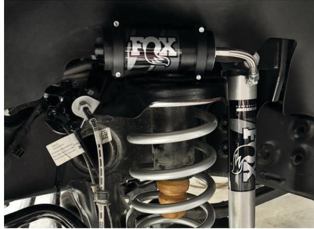
Fig. 7: Mounted Performance Series Reservoir.
