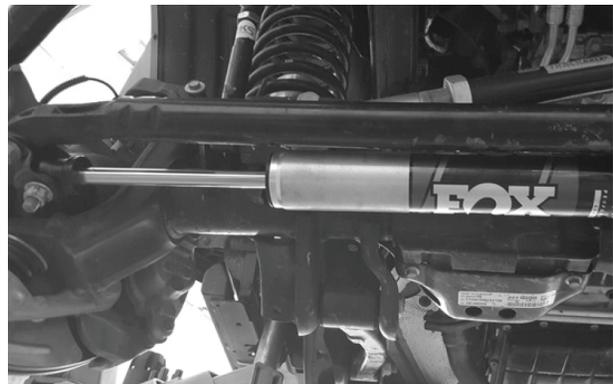
Fig. 5: Sufficient shaft clearance.
