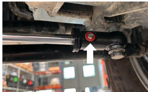
Fig. 3: Adjuster screw on eyelet.
