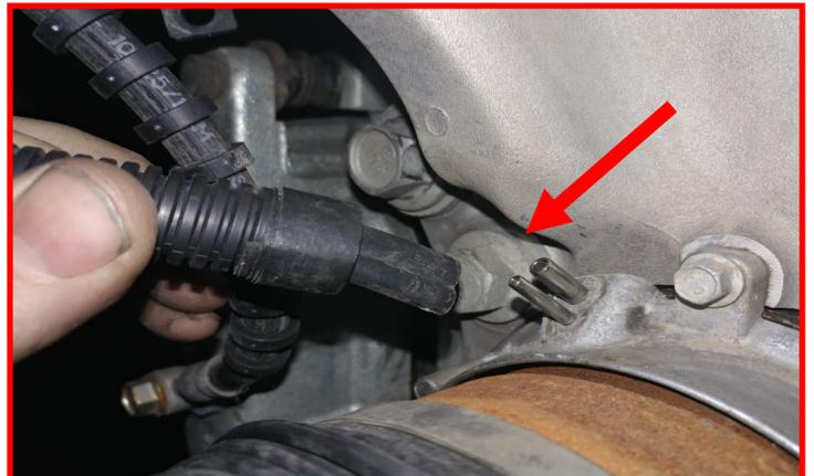
**2019 and UP Models:** Passenger side, locate the electrical harness on the coil over and follow it up onto the frame rail behind the plastic wheel liner.
