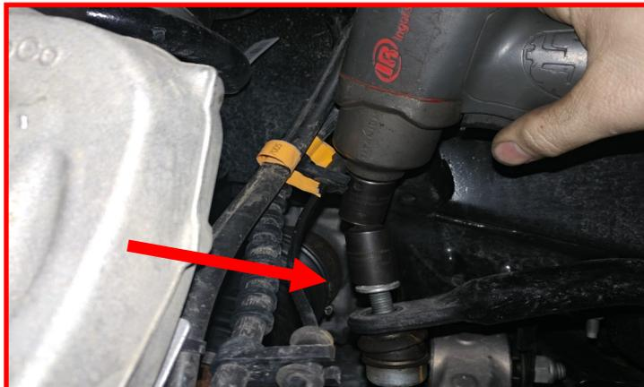
Remove the CV axle nut cover.
