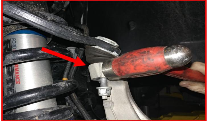
Support the lower control arm with a suitable jack. Loosen but do not remove the lower control arm bolts at the frame rail. Remove the lower coil over bolt.
