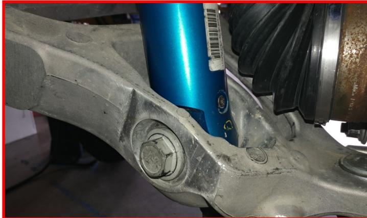
Raise the upper control arm up. Mark the frame in the center between the pocket walls  $3/4$ " down from the edge.
