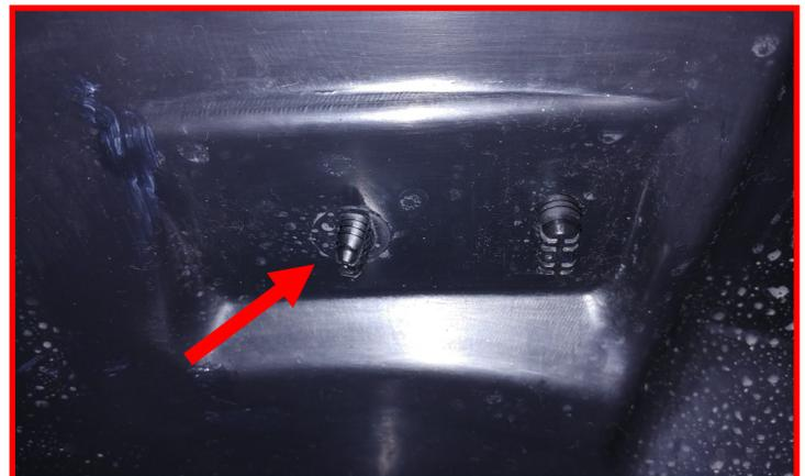
**All models:** Remove the sway bar end link from the sway bar.
