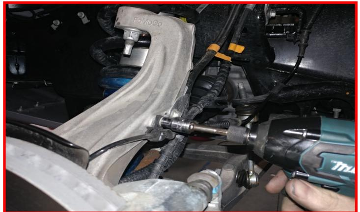
Install the sway bar end link onto the sway bar. Torque to **30 ft-lbs.**
