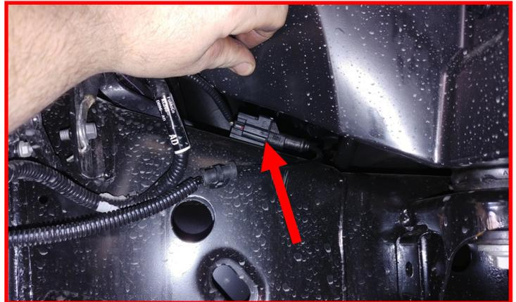
Driver side, locate the electrical harness on the coil over and follow it up onto the frame rail and into the engine bay. The wire follows the ABS harness.
