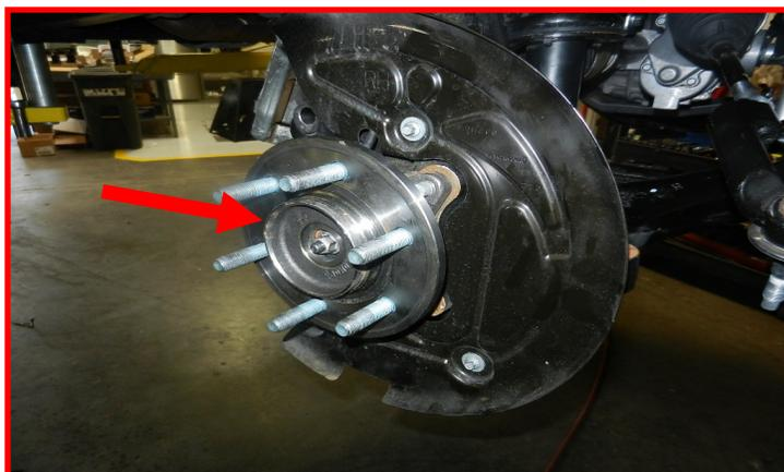
Jack the lower control arm up to add pressure to the strut. Putting a suitable jack stand at the rear of the vehicles frame will aid in keeping the load transfer from picking the front end up while jacking the lower control arm up.
