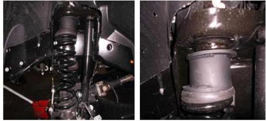
14. Install the assembly in to the vehicle. **Note: Coil Spacer position. Coil Spacer Should be orientated so the spring is offset to the front of the coil pocket and to the inside of the frame to correct "Spring Bowing"**
