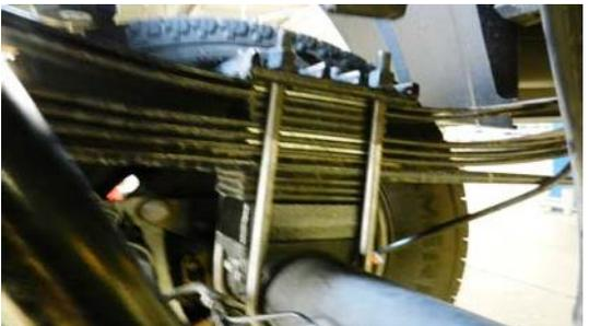
27. Install the mounting plate and longer u-bolts.
