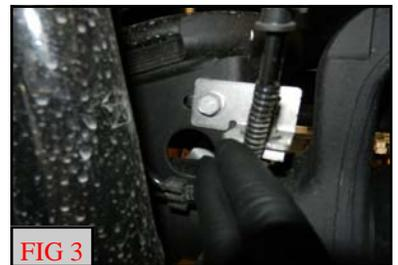
Remove the 2 brake line / ABS brackets attached to the axle. (Fig 2, 3)
