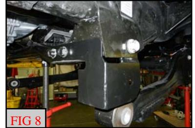
Torque the cross member bolts to **100 ft-lbs**, and the factory 18mm hardware to **200 ft-lbs**. Do not tighten the radius arms at this time.
