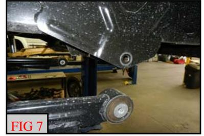
Rotate the axle and install the radius arms into the drop brackets using **18mm x 130mm bolts, washers and lock nuts**. Do not tighten at this time.
