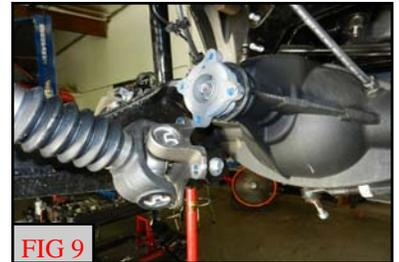
With the axle fully supported, remove the lower shock bolts.
