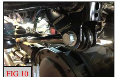
Remove the track bar at the frame and loosen at the axle. (Fig 10)
