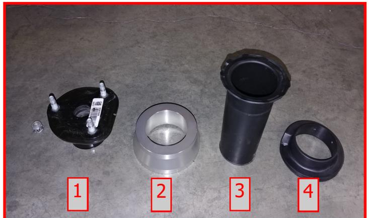
Install the ReadyLIFT preload spacer onto the dust shield/ spring seat. Install the factory top hat/rubber isolator 180 degrees from the previously made marks for orientation. This will orient the spring in its original location to prevent the spring from bowing. When tightening, make sure the top of the strut shaft is fully seated into the top hat. Torque the top strut hardware to **30 ft-lbs.**
