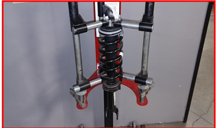
Picture shows the order of assembly for the strut: **1.** Factory top hat and rubber isolator, **2.** ReadyLIFT pre-load spacer, **3.** Factory dust shield, **4.** Factory plastic spring lock.
