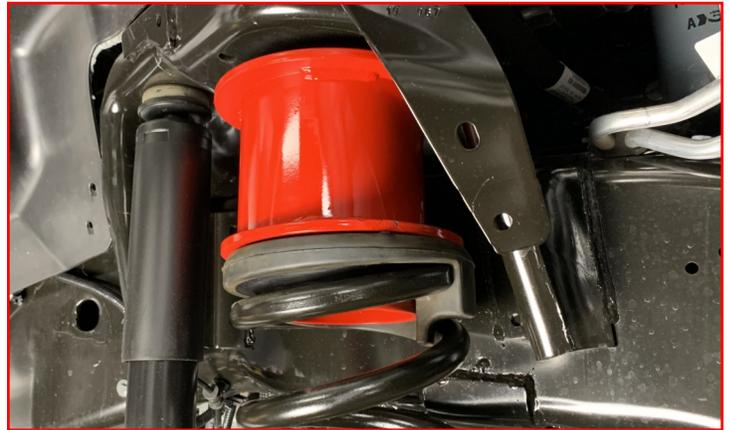
Install the supplied **shock extensions** onto the shock using **14mm bolts, washers, c-lock nuts**. Raise the axle enough to install the extension onto the axle using the **factory hardware**. Do not tighten factory hardware at this time.
