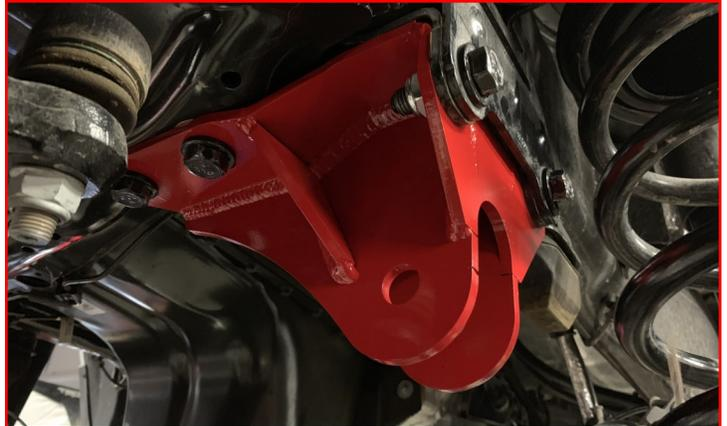
Install track bar using factory hardware. Do not tighten at this time.
