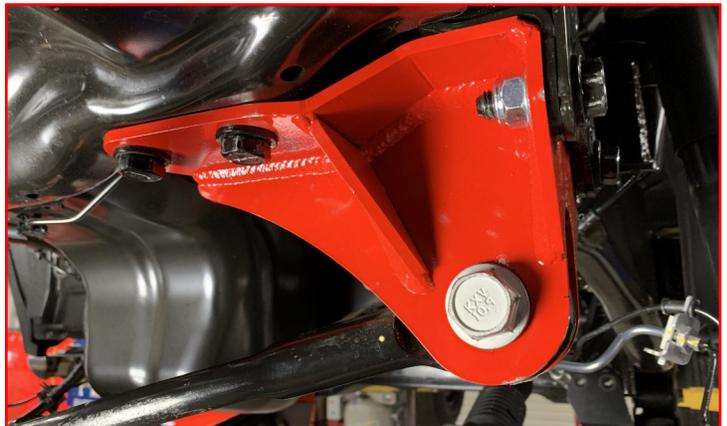
Install the **ABS sensor harness and brake line bracket** to the radius arm.
