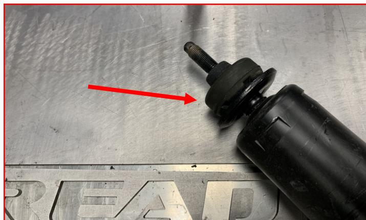
Using a liberal amount of thread locker, install the **supplied shock extensions** on to the top of the shock shaft.
