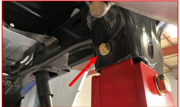
Drill hole on outside of factory track bar mount using 3/8" drill. Install the **3/8" bolts, washers and c lock nut** on the outside hole. Tighten 3/8" hardware and torque to **45 ft-lbs**. Torque the factory hardware to **100 ft-lbs**.
