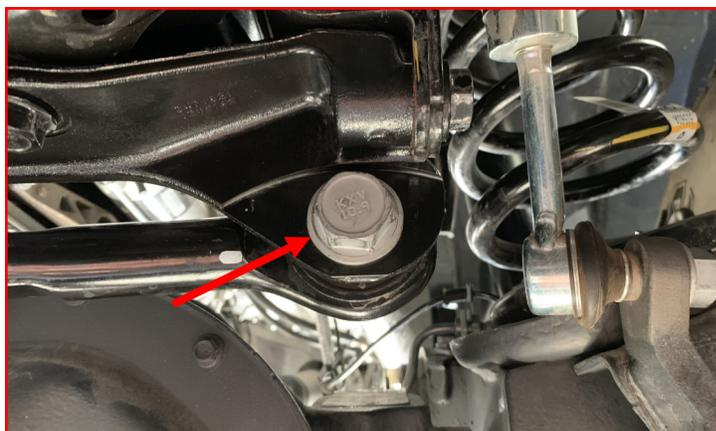
Lower the axle enough to remove the front springs. Make sure to not over extend the brake/ABS lines.
