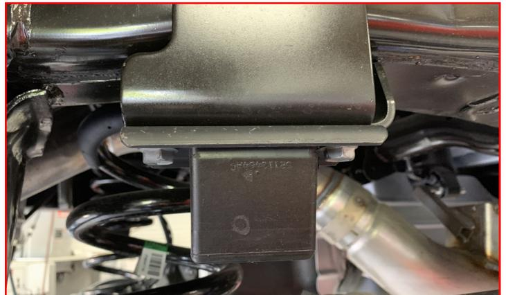
Loosen the track bar at the axle and frame mounts but do not remove.
