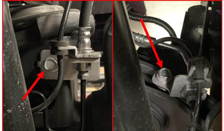
Locate the **brake line/ABS bracket** on the inside of the frame rails and remove.
