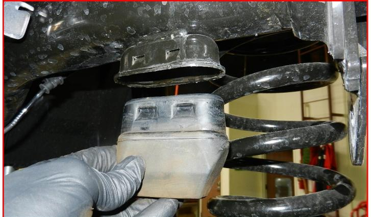
Install **extended bump stops**. To aid in install, lube the mounting end with a soap and water mix.
