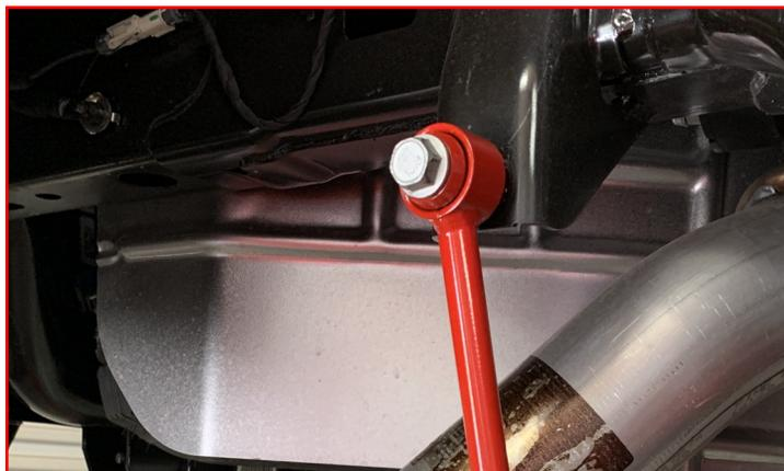
Install the sway bar end links using **M12 x 70mm bolts, washers, and c-lock nuts**. In-
