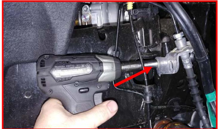
Remove the **brake line bracket** and **ABS harness** on the knuckle.
