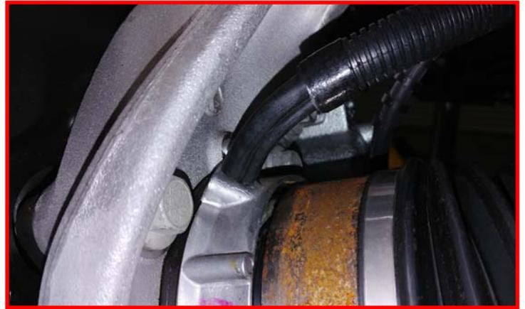
Install the brake line bracket and ABS harness to the knuckle using the **factory hardware**. Torque all to **5 ft-lbs**.
