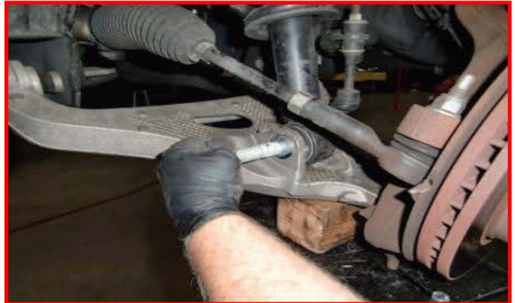
Connect the UCA to the knuckle using the **factory ball joint hardware**. Torque to **65 ft-lbs**. Install the sway bar end link to the LCA using the **factory hardware**. Torque to **35 ft-lbs**.
