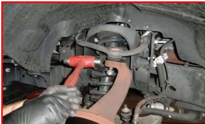
Support the lower control arm with a suitable jack. Loosen but do not remove the LCA hardware at the frame. Remove the lower strut hardware from the LCA.
