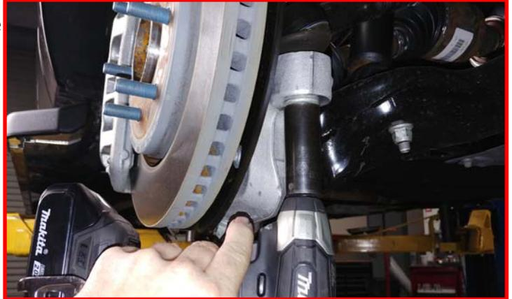
Remove upper ball joint from the knuckle. Strike the ball joint boss with a dead blow hammer to dislodge the taper.
