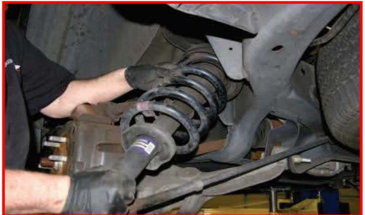
Install the ReadyLIFT strut extension to the strut using the provided **M10 flange nuts**. Torque to **30 ft-lbs**.
