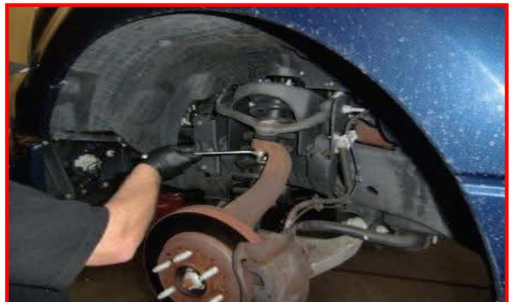
Strike the upper ball joint boss with a dead blow hammer to dislodge the taper. Remove the upper ball joint nut hardware and separate the upper control arm from the knuckle. Loosen but do not remove the upper control arm hardware.
