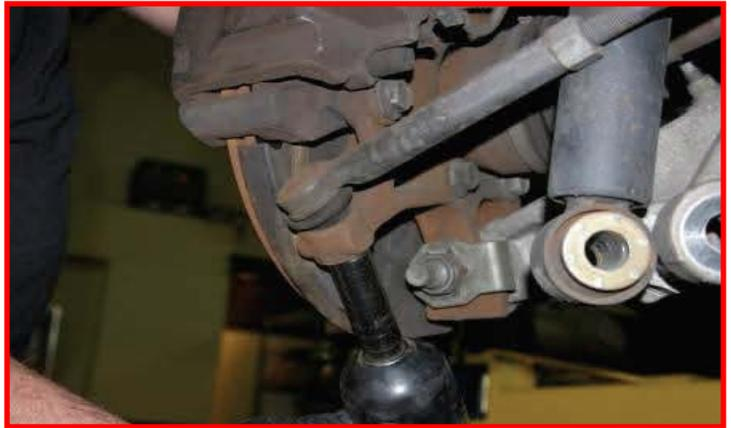
Remove the lower strut from the LCA.
