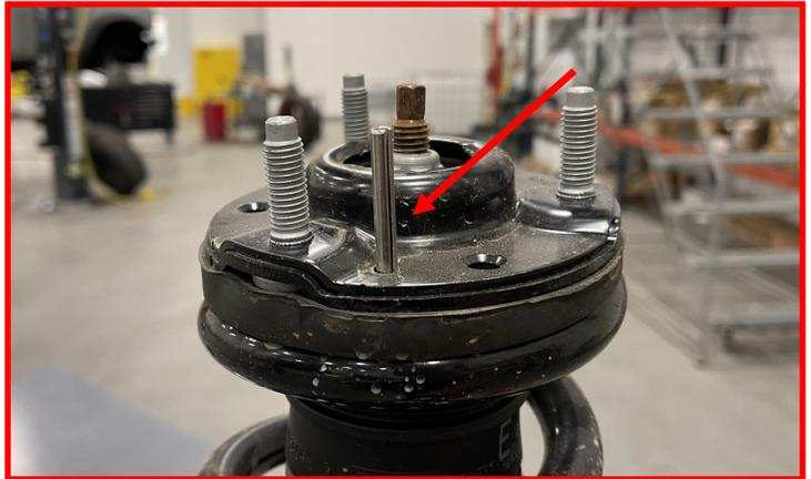
Before installing the top spacer place the strut into a spring compressor. Mark the top hat to spring location.
