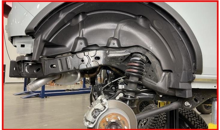
With the rear wheels removed, locate and remove the (12) mounting clips and the (3) mounting screws that hold the rear fender liners in place.
