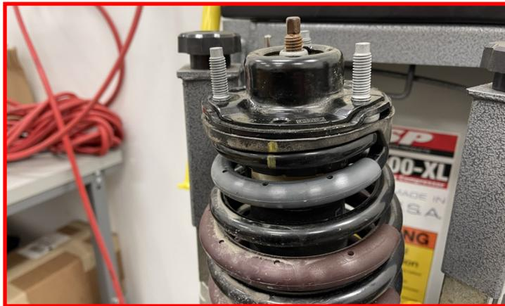
With the rear strut assembly removed from the vehicle, remove the locating pin from the top hat using pliers or similar tool.
