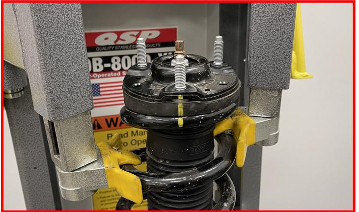
Compress the spring enough to relief pressure on the top hat. Being sure to keep the strut body and upper spring isolator in the factory location, rotate the factory top hat 180 degrees from the previously made marks. This will orient the spring in its original location to prevent the spring from bowing.
