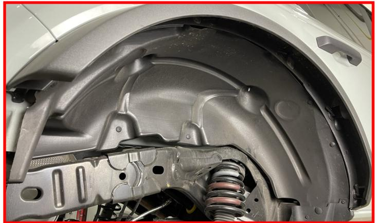
Remove the rear fender liners.
