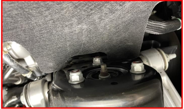
Remove the lower strut nuts.
