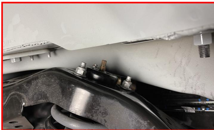
Using an appropriate jack, support the axle.
