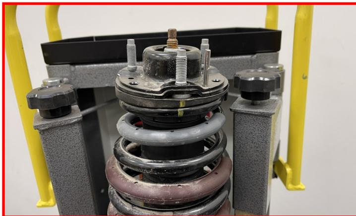
Compress the spring enough to relief pressure on the top hat. Being sure to keep the strut body and the factory spring isolator in the factory location, rotate the factory top hat 180 degrees from the previously made marks. This will orient the spring in its original location to prevent the spring from bowing.
