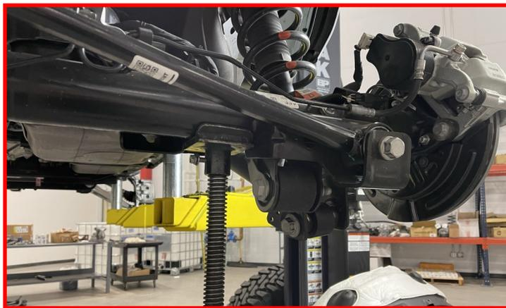
Loosen the (3) top strut nuts.
