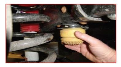
Install the ReadyLIFT bump stop spacer and factory bump stop mount using M8 x 75mm bolt and washer. Torque to 5 ft-lbs. Install the bump stop to the factory mount by pressing it back into place.
