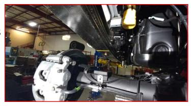
Locate the driver side lift block (Has a D cut into it under the bump stop tang). Raise the axle and the block up to the spring while aligning the center pin. Install the provided u-bolts, and nuts. Snug the u-bolt nuts but do not fully tighten at this time. Repeat steps for passenger side.
