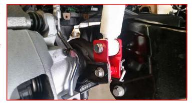
Install the ReadyLIFT brake line bracket to the factory brake line using 5/16" x .75" bolts, washers, and nuts. Install the bolt facing outwards. Gently pull the metal brake line down while lining up the ReadyLIFT bracket to the original holes in the frame. Install using factory hardware. Reattach the brake line bracket at the axle using factory hardware. Torque all to 5 ft-lbs.
