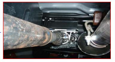
Lower the vehicle to the ground. Torque the lug nuts to the wheel manufacturers specs. Jounce the vehicle a few times to settle to the new ride height. Torque the u-bolts to 110 ft-lbs. Reattach the vehicle power source. Have a reputable alignment shop set the alignment to the factory specs.
