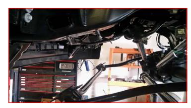
Loosen (do not remove) the radius arm bolt at the frame. Lower the axle enough to remove the front springs. Install the ReadyLIFT urethane isolator, spring spacer, and then factory rubber isolator onto the spring. Raise the axle enough to hold the spring assembly in place.
