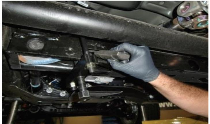
Push the torsion bar forward through the factory keyway cross member and lower control arm. You may need to use a hammer and punch on the end of the bar to break it loose from the keyway and control arm.
