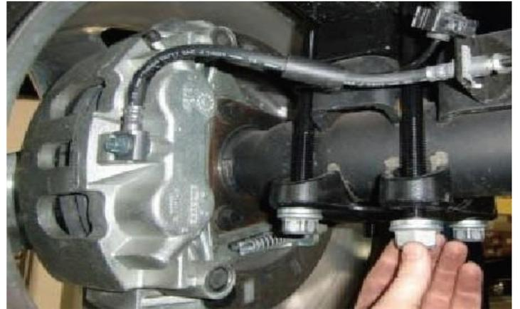
Vehicles that are not equipped with over load leaf pack may need the provided U-bolts trimmed after installation.
