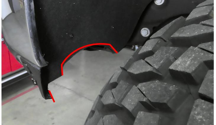
For negative offset wheels you may need to trim the plastic mud flap on the back side of the wheel. Trim the front side of the mud flap only.
