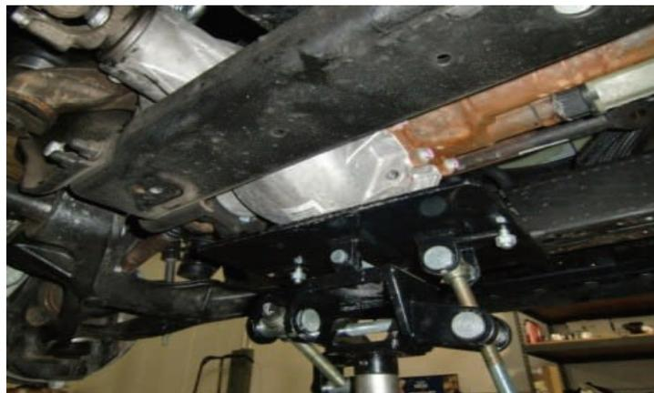
Locate the front and rear differential cradle bolts. (Total of four) Remove all and lower the differential down enough to install the differential spacers.
