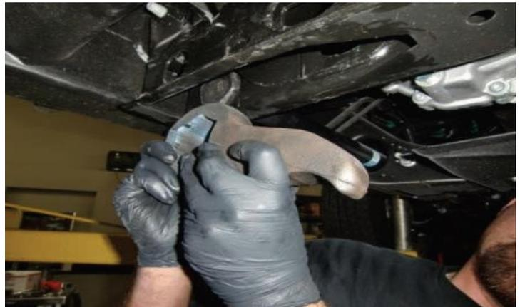
Install the ReadyLIFT keyway into the cross member while sliding the torsion bar into place. The tang of the keyway will be clocked slightly lower than the factory key. This accounts for the lift. Do not load the cross pin or bolt adjuster at this time. This will be done as one of the last steps.
