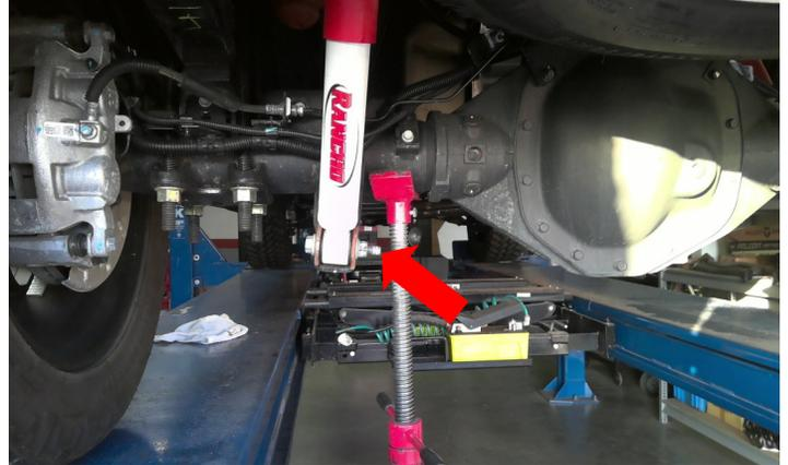
Loosen but do not remove the U-bolts on the passenger side. Remove the U-bolts completely from the driver side.
