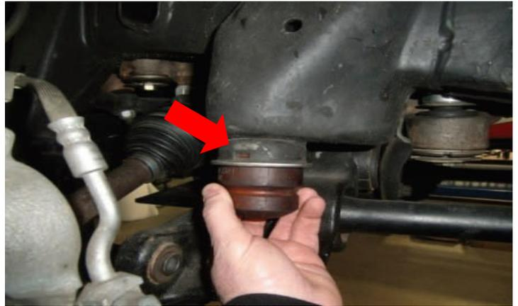
Install the ReadyLIFT bump stops. Use a soapy water solution to aid in install. You may need to use the lower control arm and a jack to "press" them into place.
