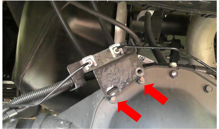
Support the axle with a suitable jack. Remove the driver and passenger shocks. Retain hardware and shocks.
